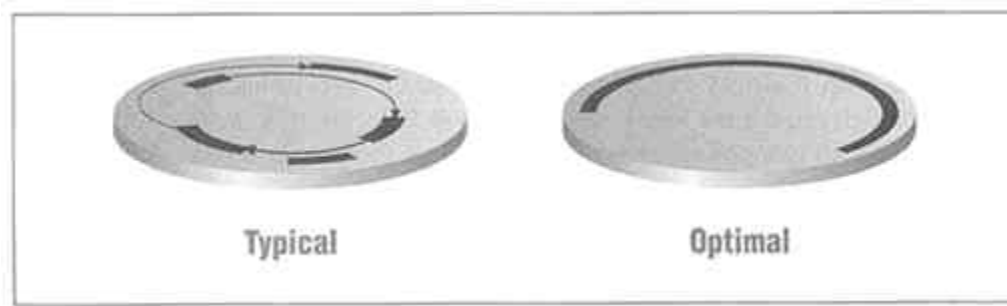
Figure 6-1. Normal UNIX disk layout and optimal layout for sequential access
