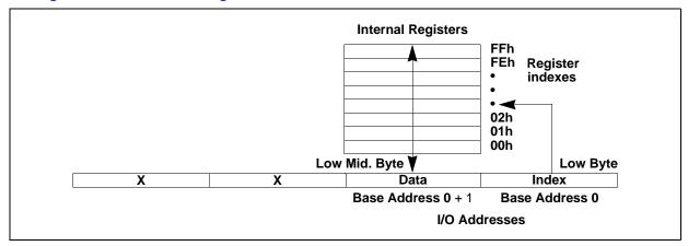
Figure 9. Indexed 8-Bit Register Example
