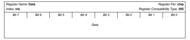
The **Data** register is accessed at **Base Address 0** + 1. This register indicates the contents of the register at the Socket/Register Index selected by the Index register.
