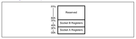
When viewed as a 7-bit value, the contents of this register completely specify a single internal-register byte. For example, when the value of this register is in the range 00h–3Fh, a Socket A register is selected (Socket Index bit is a '0'), and when the value of this register is in the range 40h–7Fh, a Socket B register is selected (Socket Index bit is a '1').
