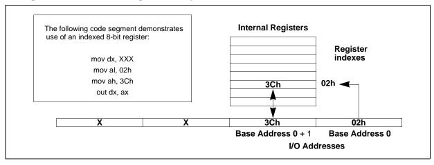
The PD6729 has Extension registers that add to the functionality of the 82365SL-compatible register set. Within the Extension registers is an **Extended Index** register and **Extended Data** register that provide access to more registers. The registers accessed through **Extended Index** and **Extended Data** are thus double indexed. The example below shows how to access the **Extension Control 1** register, one of the double-indexed registers.
