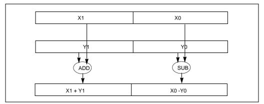
Figure 12-1. Asymmetric Processing in ADDSUBPD
