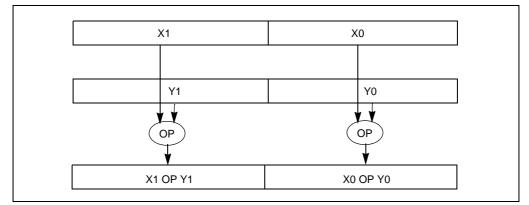
Figure 11-3. Packed Double-Precision Floating-Point Operations
