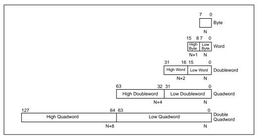
Figure 4-1. Fundamental Data Types
