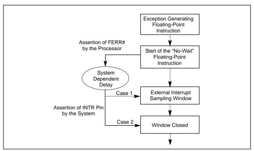
Figure D-3. Timing of Receipt of External Interrupt
