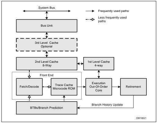
Figure 2-2. The Intel NetBurst Microarchitecture
