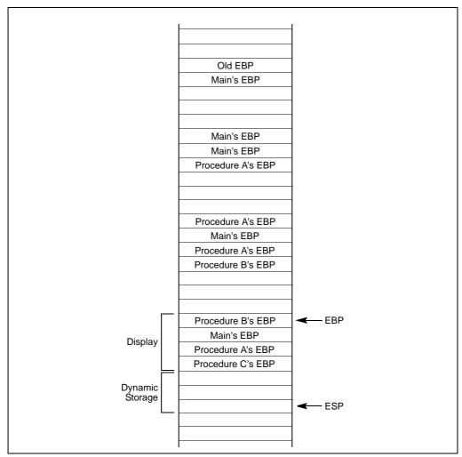
Figure 6-10. Stack Frame After Entering Procedure C
