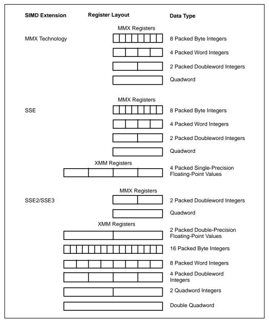
Figure 2-3. SIMD Extensions, Register Layouts, and Data Types
