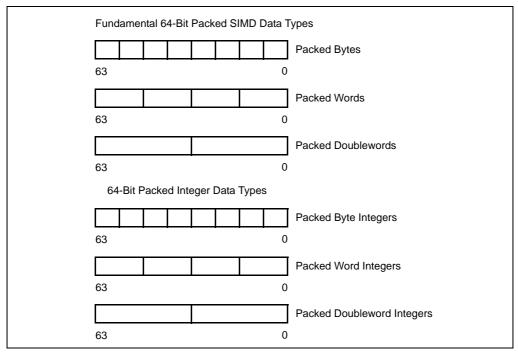
Figure 4-7. 64-Bit Packed SIMD Data Types
