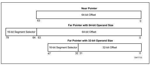
Figure 4-5. Pointers in 64-Bit Mode
