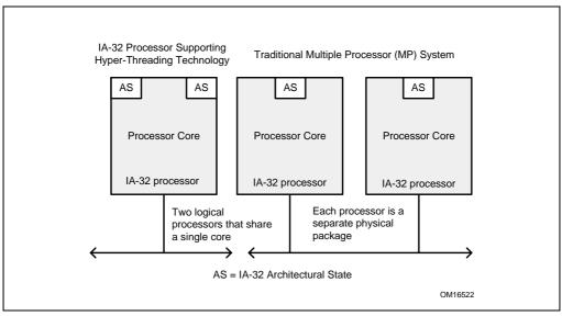
Figure 2-4. Comparison of an IA-32 Processor Supporting Hyper-Threading Technology and a Traditional Dual Processor System
