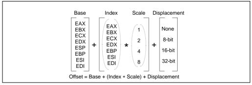
Figure 3-11. Offset (or Effective Address) Computation
