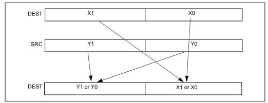
Figure 11-5. SHUFPD Instruction, Packed Shuffle Operation
