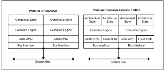
Figure 2-5. IA-32 Processors that Support Dual-Core
