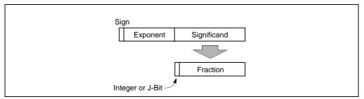
Figure 4-11. Binary Floating-Point Format
