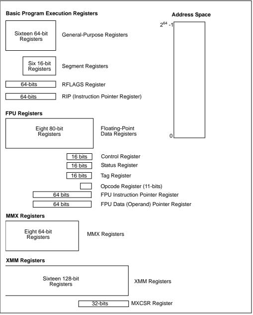
Figure 3-2. 64-Bit Mode Execution Environment
