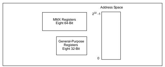
Figure 9-1. MMX Technology Execution Environment
