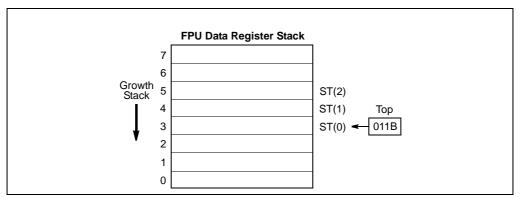
Figure 8-2. x87 FPU Data Register Stack
