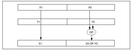
Figure 11-4. Scalar Double-Precision Floating-Point Operations
