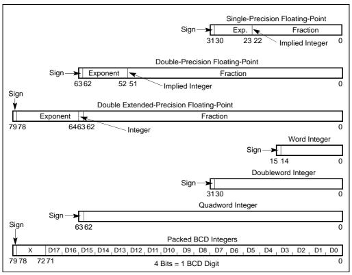
Figure 8-13. x87 FPU Data Type Formats
