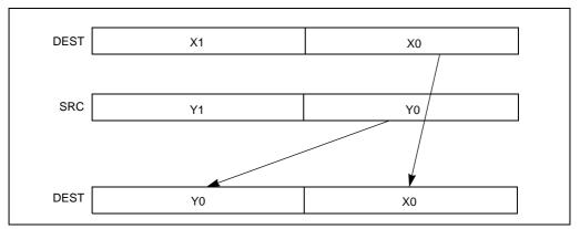
Figure 11-7. UNPCKLPD Instruction, Low Unpack and Interleave Operation
