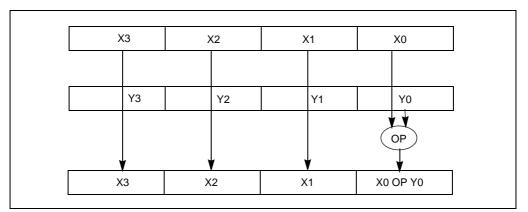
Figure 10-6. Scalar Single-Precision Floating-Point Operation
