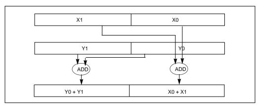
Figure 12-2. Horizontal Data Movement in ADDSUBPD
