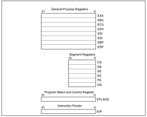
Figure 3-4. General System and Application Programming Registers
