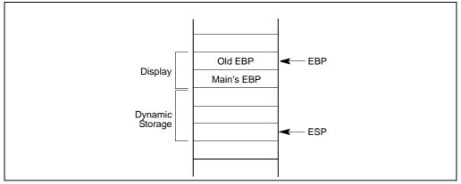
Figure 6-7. Stack Frame After Entering the MAIN Procedure
