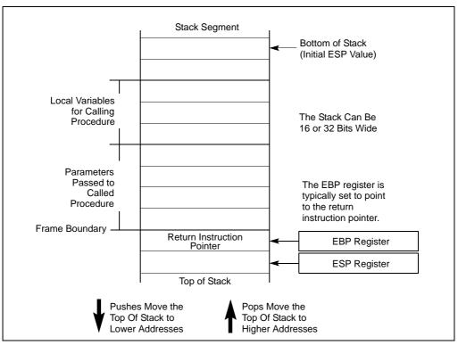
Figure 6-1. Stack Structure
