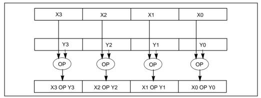
Figure 10-5. Packed Single-Precision Floating-Point Operation
