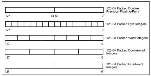
Figure 11-2. Data Types Introduced with the SSE2 Extensions
