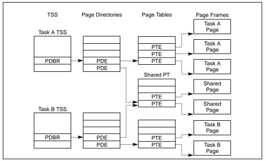
Figure 6-9. Overlapping Linear-to-Physical Mappings
