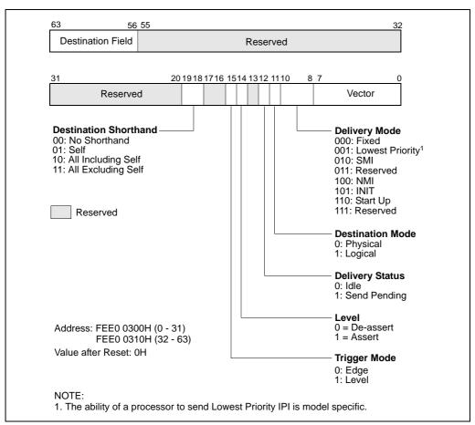
Figure 8-12. Interrupt Command Register (ICR)
