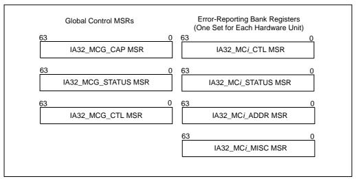
Figure 14-1. Machine-Check MSRs
