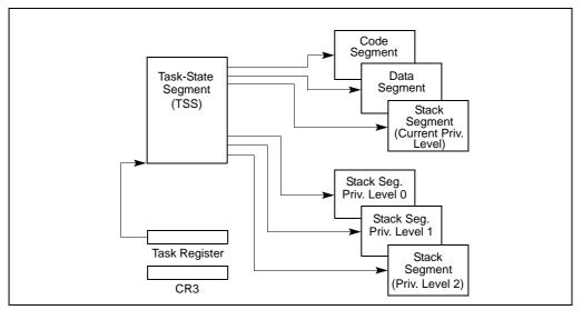
Figure 6-1. Structure of a Task
