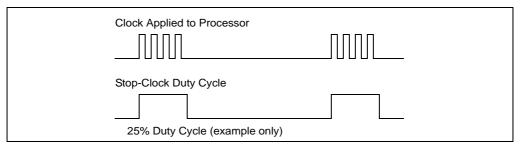
Figure 13-1. Processor Modulation Through Stop-Clock Mechanism
