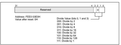
Figure 8-10. Divide Configuration Register
