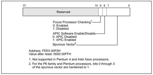
Figure 8-23. Spurious-Interrupt Vector Register (SVR)
