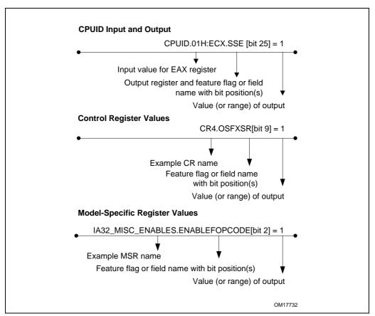
Figure 1-2. Syntax for CPUID, CR, and MSR Data Presentation
