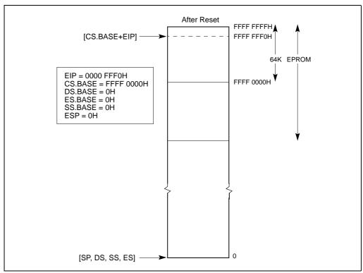
Figure 9-3. Processor State After Reset
