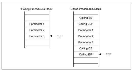
Figure 4-13. Stack Switching During an Interprivilege-Level Call
