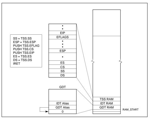
Figure 9-6. Task Switching (Lines 282-296 of List File)
