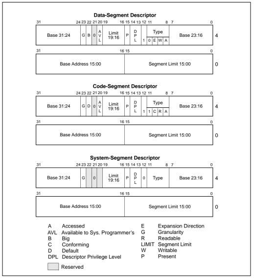
Figure 4-1. Descriptor Fields Used for Protection
