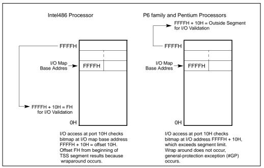
Figure 17-1. I/O Map Base Address Differences
