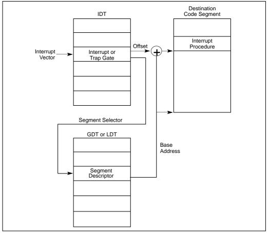
Figure 5-3. Interrupt Procedure Call
