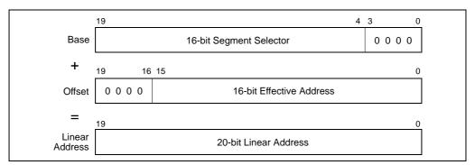
Figure 15-1. Real-Address Mode Address Translation
