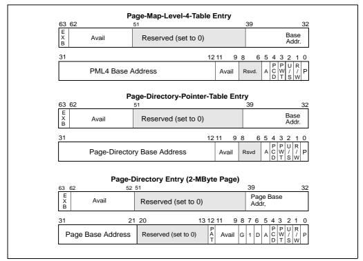
Figure 3-27. Format of Paging Structure Entries for 2-MByte Pages in IA-32e Mode
