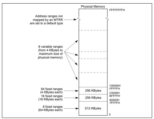
Figure 10-3. Mapping Physical Memory With MTRRs
