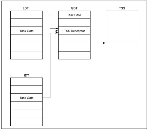
Figure 6-7. Task Gates Referencing the Same Task
