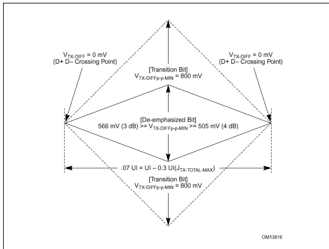
There are two eye diagrams that must be met for the transmitter. Both eye diagrams must be aligned in time using the jitter median to locate the center of the eye diagram. The different eye diagrams will differ in voltage depending whether it is a transition bit or a de-emphasized bit.
