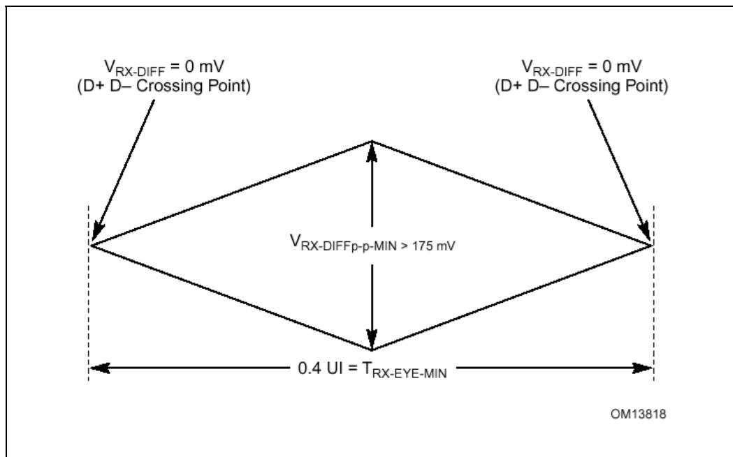
The RX eye diagram must be aligned in time using the jitter median to locate the center of the eye diagram. The eye diagram must be valid for any 250 consecutive UIs. An appropriate average TX UI must be used as the interval for measuring the eye diagram.
