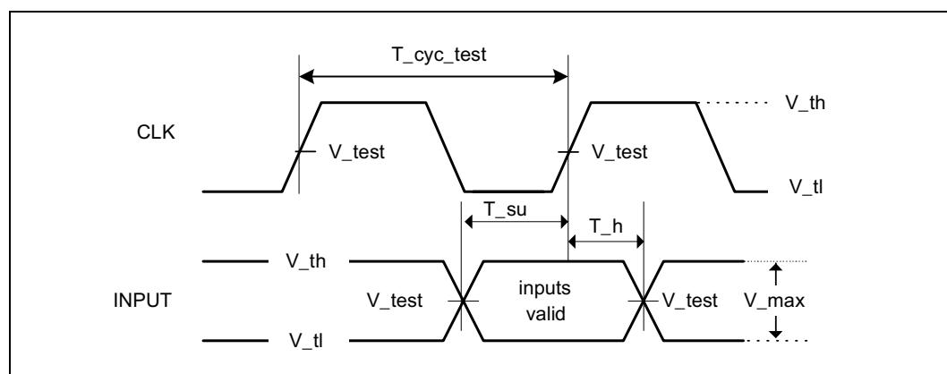
**Table 17. PCI-X 3.3V Signal Timing Parameters**
