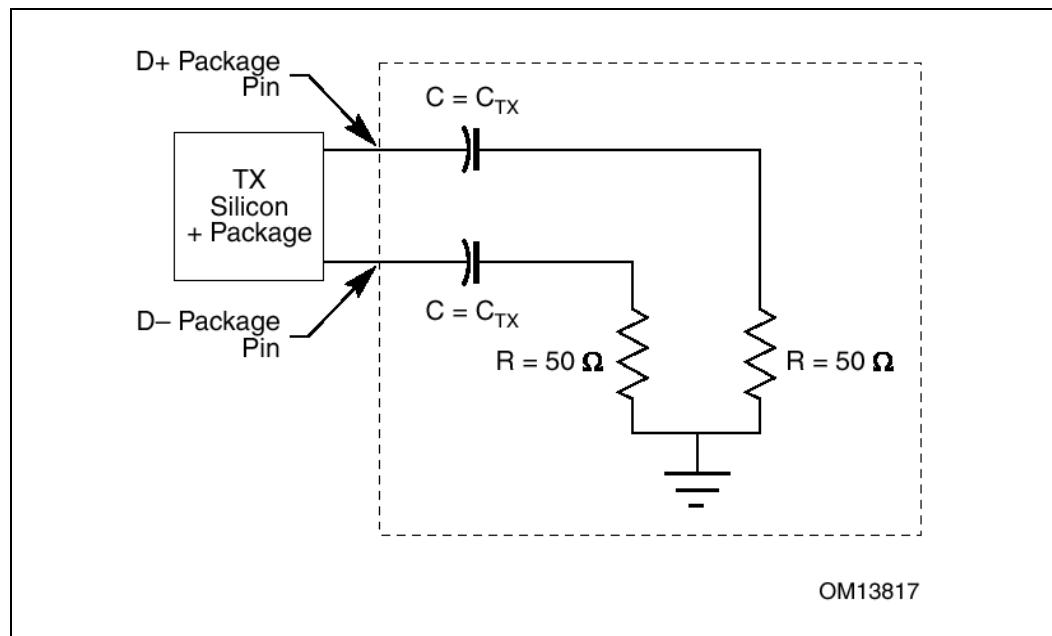
The test load is shown at the transmitter package reference plane, but the same Test/Measurement load is applicable to the receiver package reference plane. CTX is an optional portion of the measurement test load. The measurement should be taken on the opposite side of the capacitor from the package, and the value of the CTX must be in the range of 75 nF to 200 nF.
