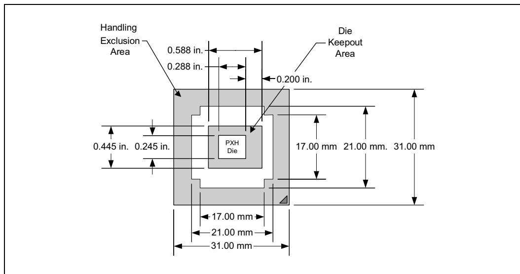
**Figure 10.** 41210 Bridge Package Dimensions (Side View)
