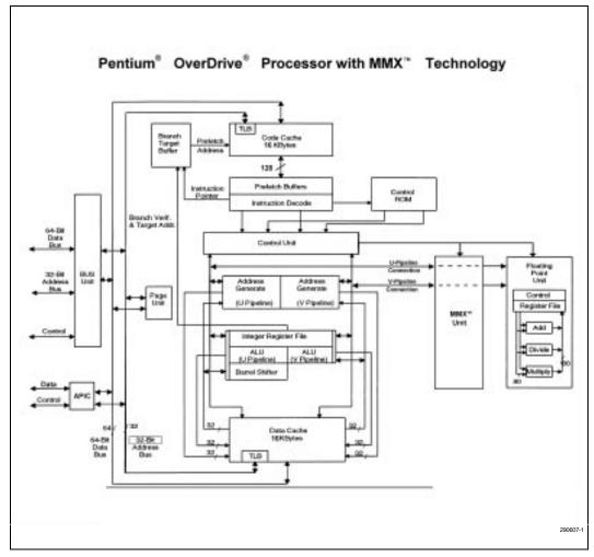
Figure 1. Pentium<sup>®</sup> OverDrive<sup>®</sup> Processor with MMX™ Technology Block Diagram
