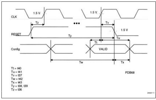
Figure 11. Reset and Configuration Timing
