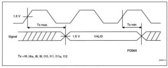
Figure 8. Valid Delay Timing
