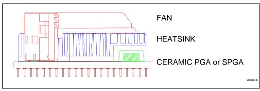
Figure 6. Pentium® OverDrive® Processor with MMX™ Technology with Fan/Heatsink
