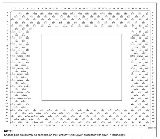
Figure 18. Pentium® OverDrive® Processor with MMX™ Technology Pinout—Top Side View
