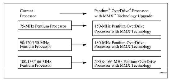
Figure 3. Pentium® OverDrive® Processor with MMX™ Technology Upgrade Choices
