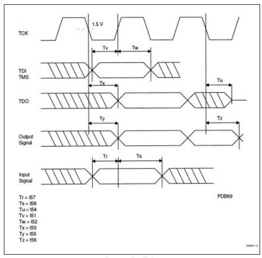
Figure 12. Test Timing
