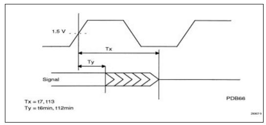
Figure 9. Float Delay Timing
