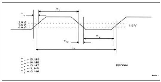
Figure 7. Clock Waveform
