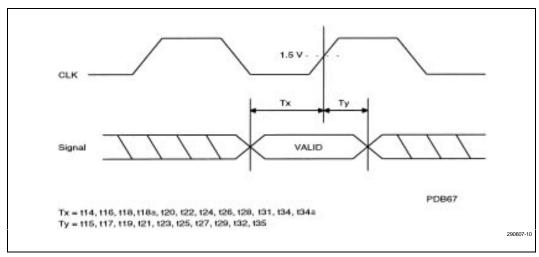
Figure 10. Setup and Hold Timing
