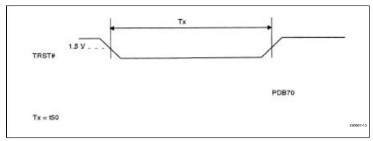
Figure 13. Reset and Configuration Timing
