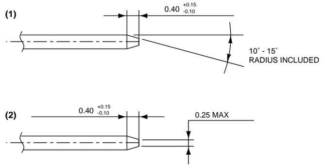
**PIN-CONNECTOR PIN-TIP FORM AND DIMENSIONS ((1) or (2))**
