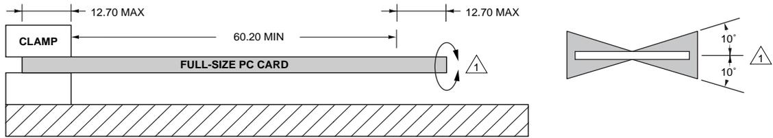
△ APPLY TORQUE TO UNCLAMPED END OF PC CARD. THE TORQUE AND ANGLE MAX ARE:
