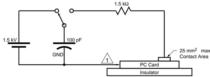
1 Connect to the four (4) ground contacts (Pin No' s 1, 34, 35 and 68)
