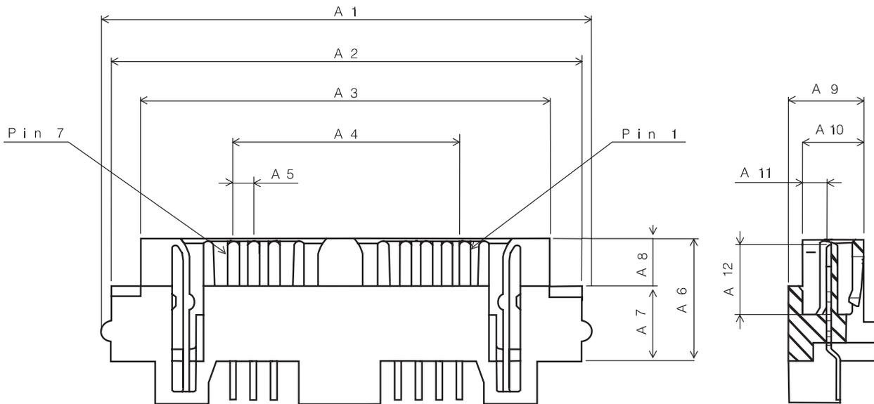
Figure 3-8: Card I/O Connector, 7 Position
