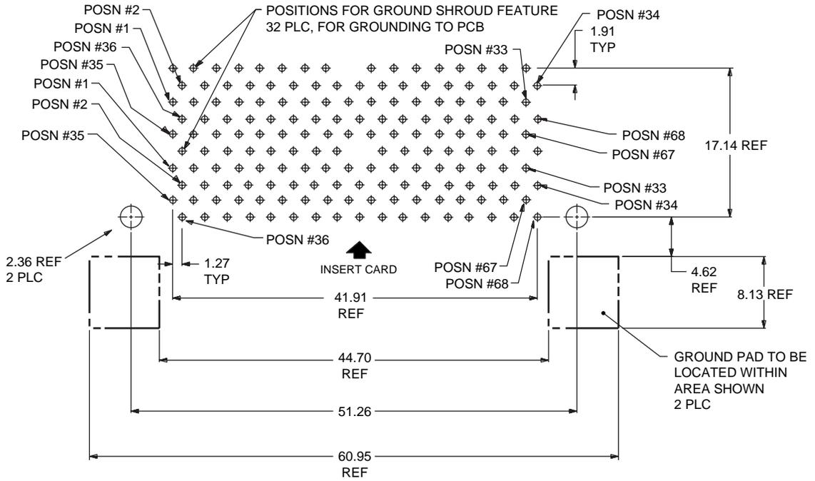
Figure 11-44: CardBus PC Card Recommended Right Angle PCB Footprint (Stacked)
