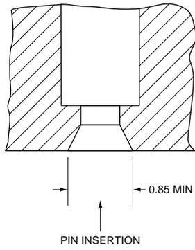
**Figure 11-12: Small PC Card Connector Socket**
