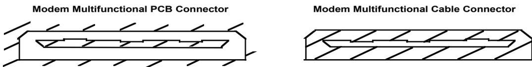
Figure 3-6: Reserved Connector Key Configuration
