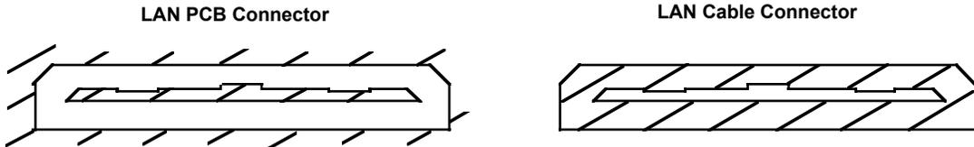
Figure 3-4: Open Standard LAN Connector Key Configuration
