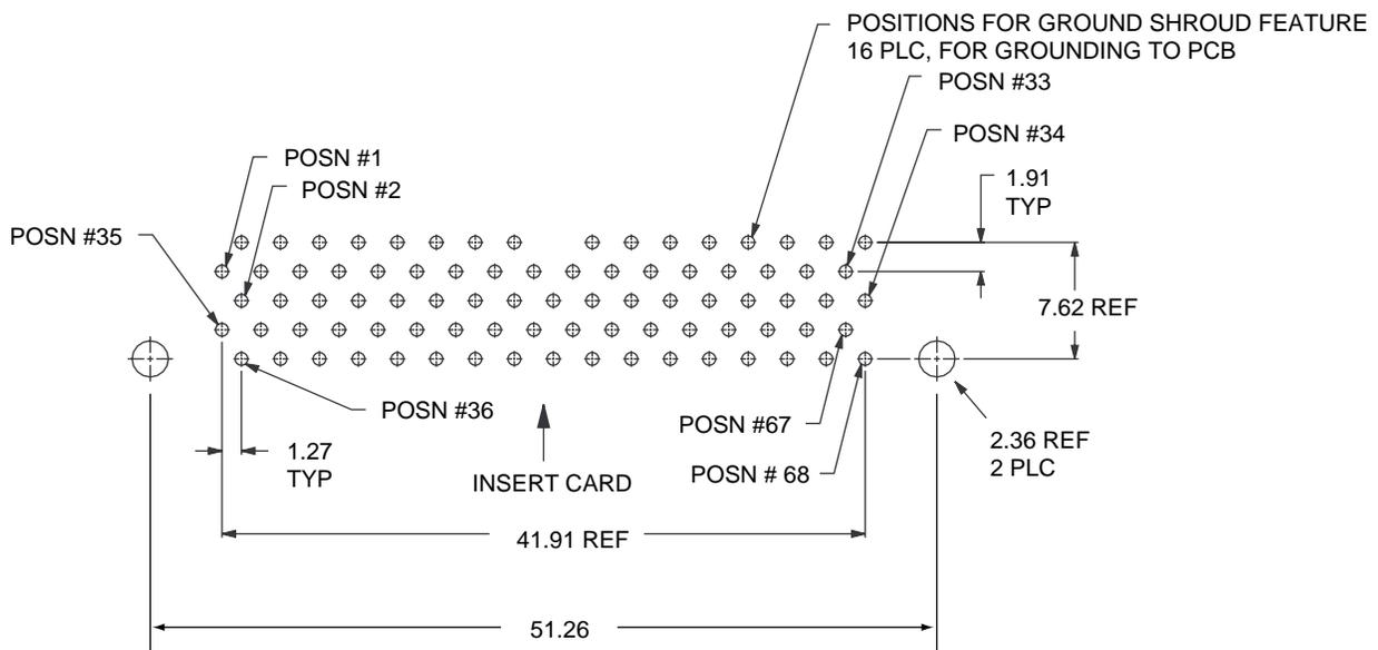
**Figure 11-43: CardBus PC Card Recommended Right Angle PCB Footprint**
