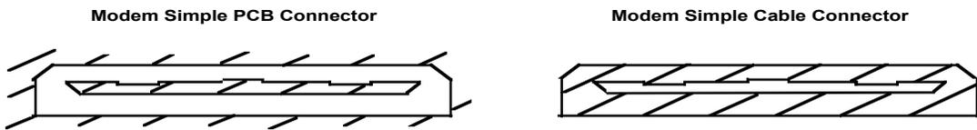
Figure 3-5: Reserved Connector Key Configuration
