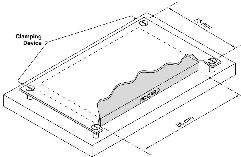
1. The PC Card shock and vibration test fixture shall entrap the PC Card such that all shock and vibration shall be transmitted into the sample card
