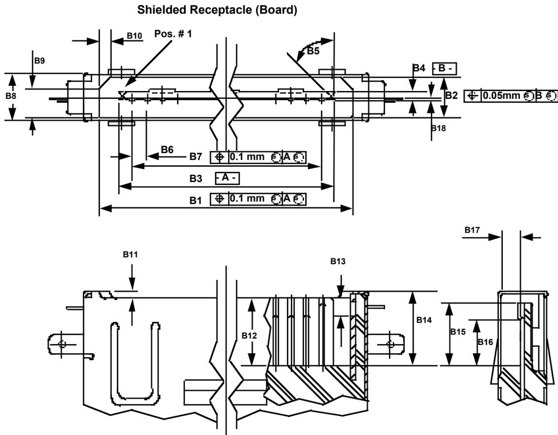
Figure 3-1: PCB Connector
