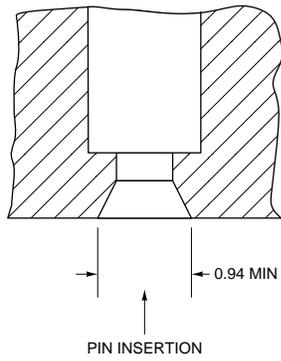
**Figure 11-11: Full-size PC Card Connector Socket**
