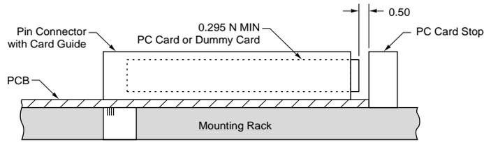
**Figure 11-25: Connector Shock & Vibration Test Fixture**
