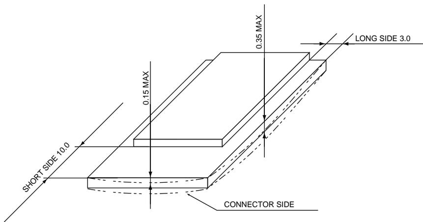
Figure 11-33: Warpage Measurement A-Interconnect Area
