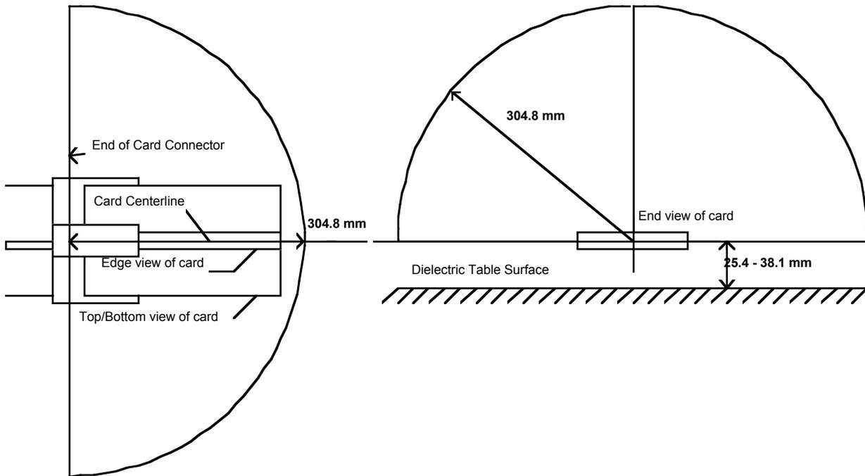
**Figure 10-2: Free Area Around Card Being Rated**
