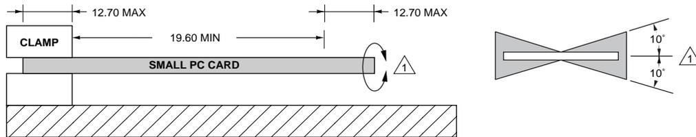
△ APPLY TORQUE TO UNCLAMPED END OF SMALL PC CARD. THE TORQUE AND ANGLE MAX ARE:
