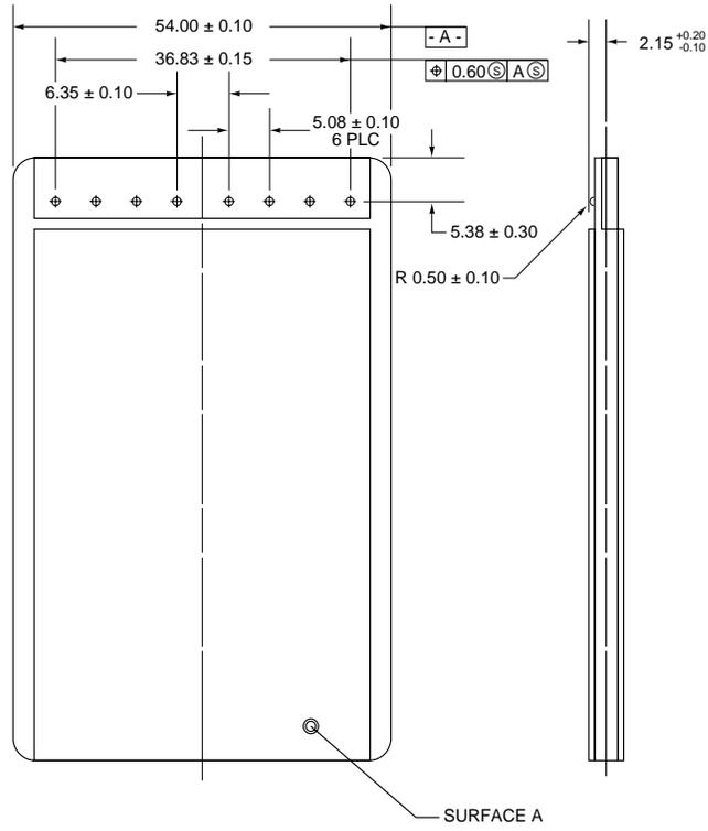
Figure 11-40: CardBus PC Card Recommended Connector Grounding Interface Dimensions
