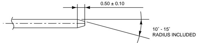
**PIN-CONNECTOR PIN-TIP FORM AND DIMENSIONS**
