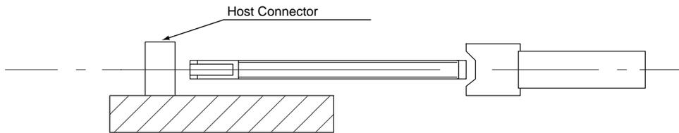
**Figure 11-39: Card Inverse Insertion Push Block**
