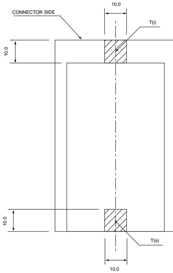
Figure 11-35: Warpage Measurement B-Thickness Measurements
