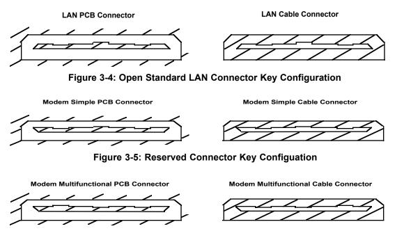
Figure 3-6: Reserved Connector Key Configuration
