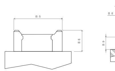
Figure 3-10: Cable Plug Connector, 4 Position
