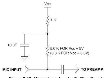
Figure 3-12: Microphone Input with Bias Supply
