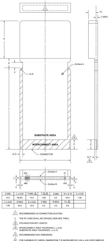
6 FOR CARDBUS PC CARDS, DIMSENTION T IS INCREASED BY 0.50 ± 0.05 OVER DIMPLES (REFER TO CARDBUS PC CARD RECOMMENDED CONNECTOR GOUNDING INTERFACE DIMENSIONS FIGURE IN THE PHYSICAL SPECIFICATION)
