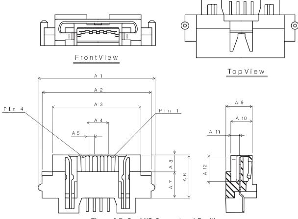
Figure 3-7: Card I/O Connector, 4 Position
