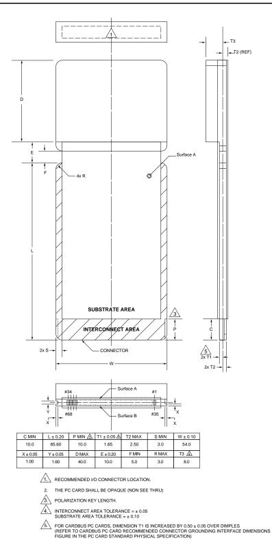
Figure 3-16: Type II Extended PC Card Package Dimensions
