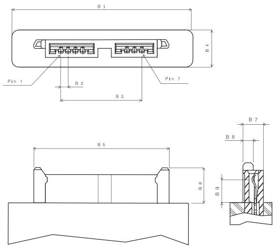
Figure 3-11: Cable Plug Connector, 7 Position
