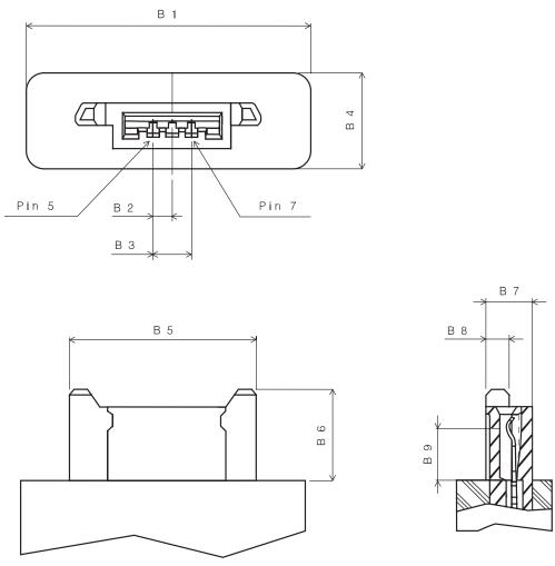
Figure 3-9: Cable Plug Connector, 3 Position
