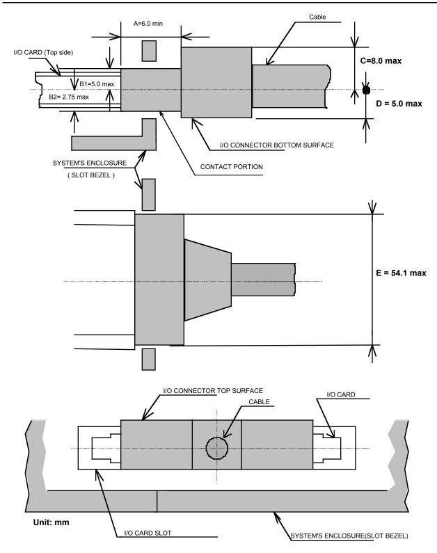
Figure 3-13: Maximum Dimensions for I/O Connector
