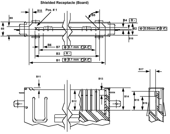
Figure 3-1: PCB Connector
