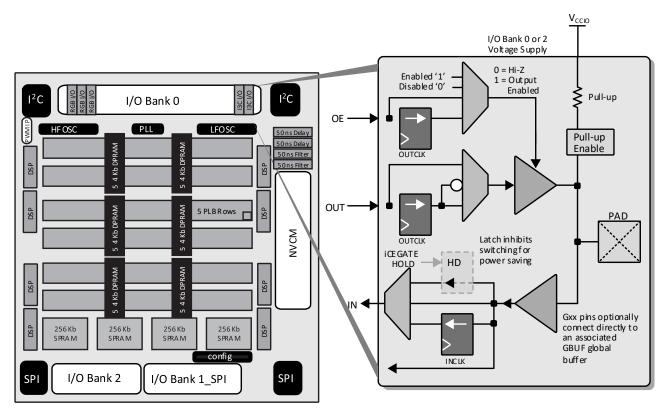
Figure 3.9. I/O Bank and Programmable I/O Cell
