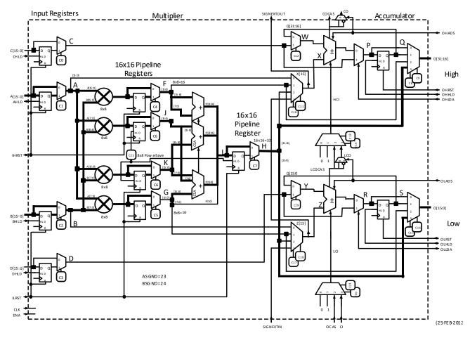
Figure 3.8. DSP 16-bit x 16-bit Multiplier
