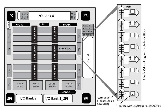
Figure 3.1. iCE40UP5K Device, Top View
