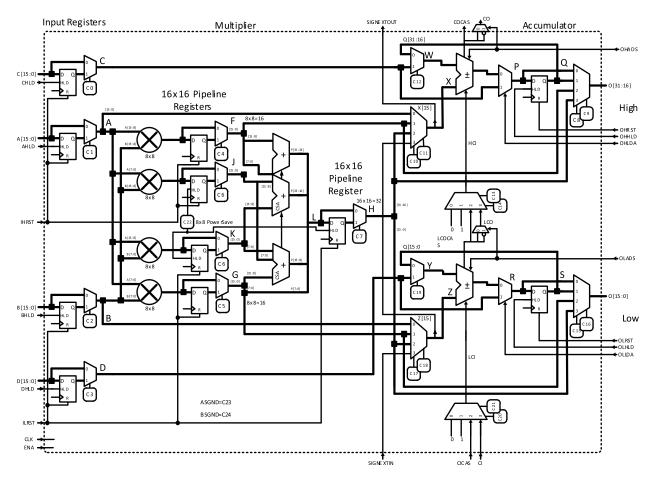
Figure 3.6. sysDSP Functional Block Diagram (16-bit x 16-bit Multiply-Accumulate)
