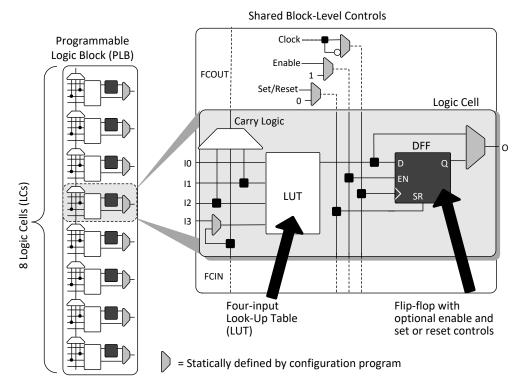
Figure 3.2. PLB Block Diagram
