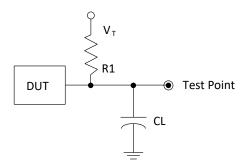
Figure 4.3. Output Test Load, LVCMOS Standards
