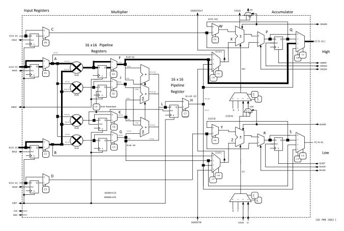
Figure 3.7. sysDSP 8-bit x 8-bit Multiplier
