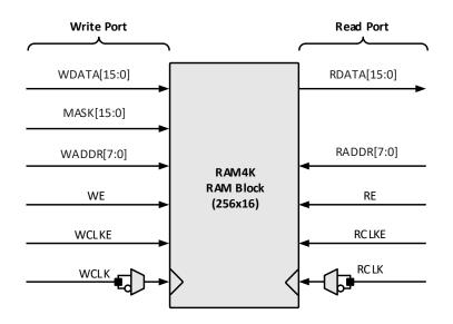
Figure 3.4. sysMEM Memory Primitives
