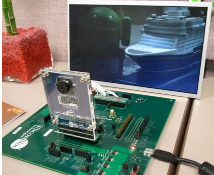
Figure 11.3. 5-Megapixel CMOS Camera to LVDS Display on iCEman40 Evaluation Board
