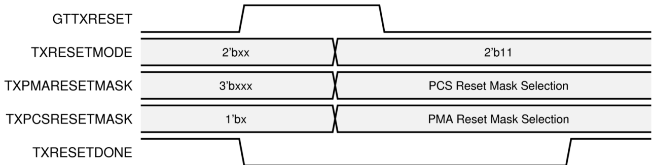
Figure 19: Transmitter Reset after GTTXRESET Pulse in Component Single Mode
