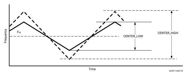
Figure 45: Center-Spread Modulation (CENTER\_LOW vs. CENTER\_HIGH)
