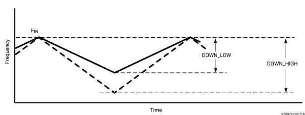
Figure 46: Down-Spread Modulation
