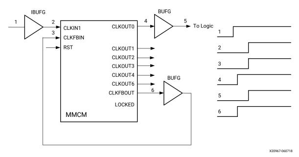
Figure 36: Global Clock Network Deskew Using Two BUFGs
