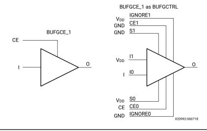
**IMPORTANT!** The select signal must meet the setup time requirement because the clock enable line uses the CE pin of the BUFGCTRL. Violating this setup time can result in a glitch.
