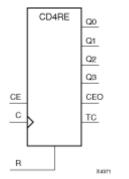
Macro: 4-Bit Cascadable BCD Counter with Clock Enable and Synchronous Reset
