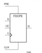
Primitive: D Flip-Flop with Clock Enable and Asynchronous Preset and Clear
