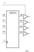
Macro: 4-Bit D Flip-Flop with Active-Low 3-State Output Buffers
