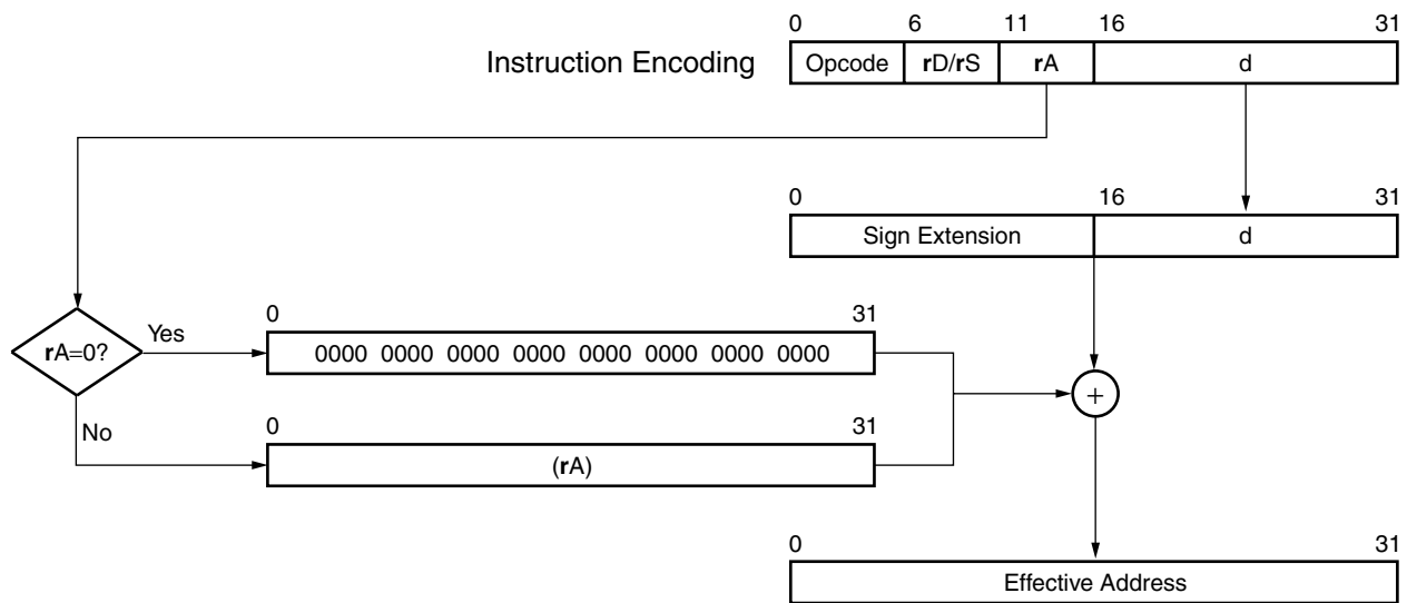
Figure 3-17: Register-Indirect with Immediate-Index Addressing
