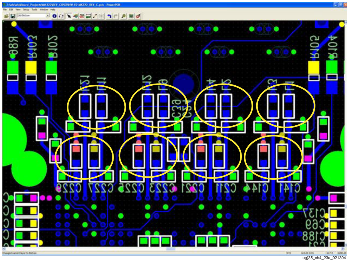
Figure 4-23: Example Power Filtering PCB Layout for Four MGTs (In Device With Internal Capacitors), Bottom Layer
