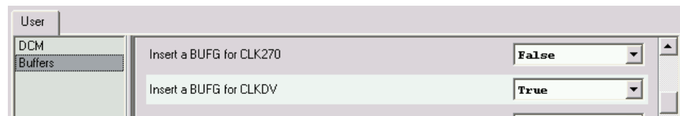
Figure 10: Configuration Window: Insert a Clock Buffer
