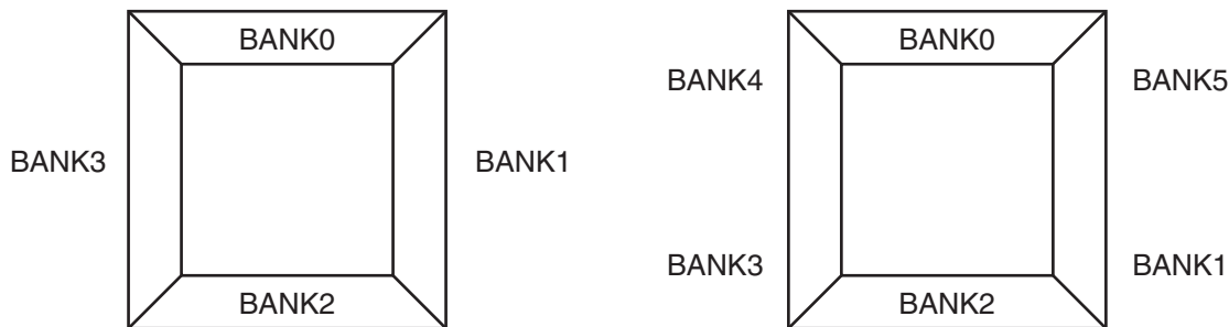
Figure 1-3: Spartan-6 FPGA I/O Banks
