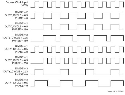
Figure 3-8: Output Counter Clock Synthesis Examples
