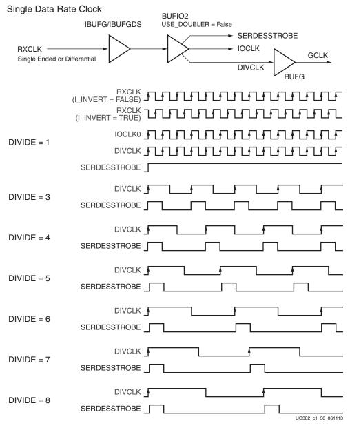
Figure 1-32: BUFIO2 Single Data Rate Clock
