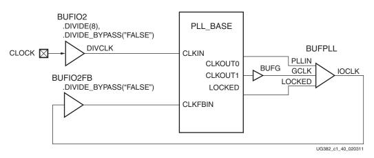
Figure 1-41: Dividing Clocks Using BUFIO2 and BUFIO2FB
