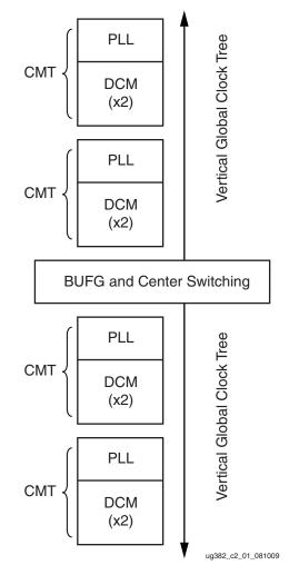
Figure 2-1: Spartan-6 FPGA CMT Location
