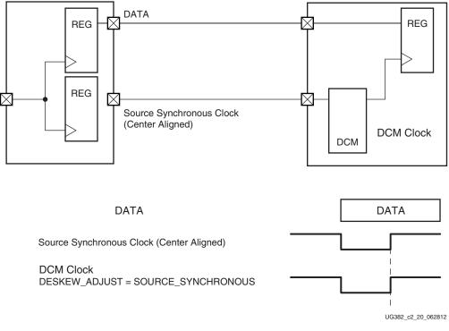
uses the shortest skew adjustment to balance the setup time with the hold time for the input register.
