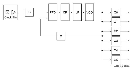
Figure 3-2: Block Diagram of the Spartan-6 FPGA PLL
