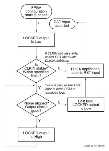
Figure 2-10: Functional Behavior of LOCKED Output
