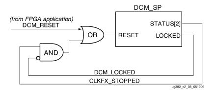
Figure 2-11: Spartan-6 FPGA DCM DFS Lock Logic
