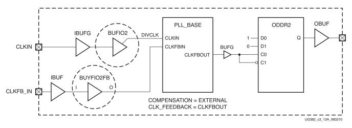
Figure 3-13: Zero Delay Buffer for Single-Ended Clocks
