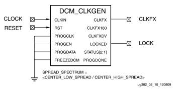
Figure 2-16: Fixed Spread Spectrum
