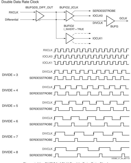
Figure 1-36: BUFIO2\_2CLK Double Data Rate Clock
