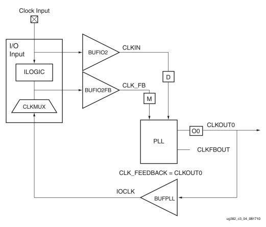
Figure 3-5: PLL Using CLKOUT0 Feedback
