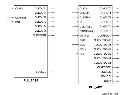
The two Spartan-6 FPGA PLL primitives, PLL\_BASE and PLL\_ADV, are shown in Figure 3-6.
