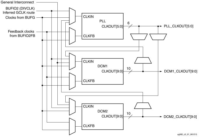
Figure 3-1: Block Diagram of the Spartan-6 FPGA CMT
