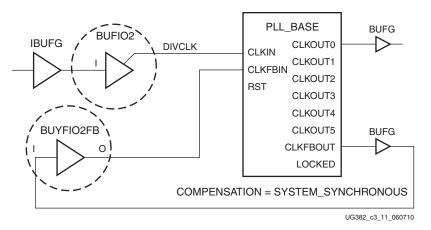
Figure 3-11: Clock Deskew Using Two BUFGs
