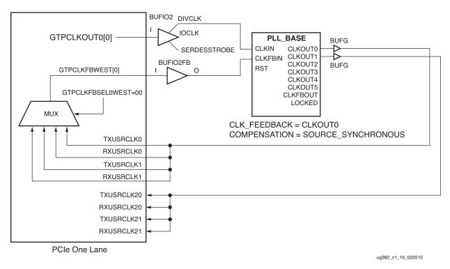
Figure 1-19: Example 6: Single Lane Clocking for PCI Express
