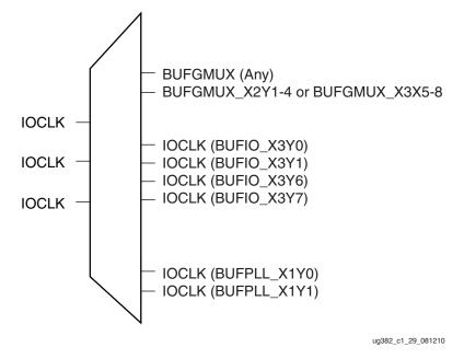
An example of the I/O clock network routing for the three I/O clocks is described in Figure 1-30.
