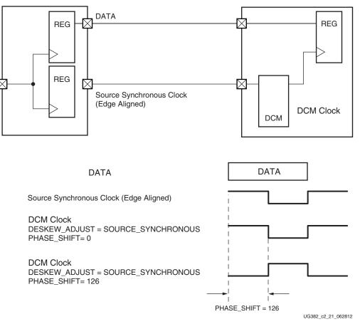
Figure 2-5: Source Synchronous Edge Aligned
