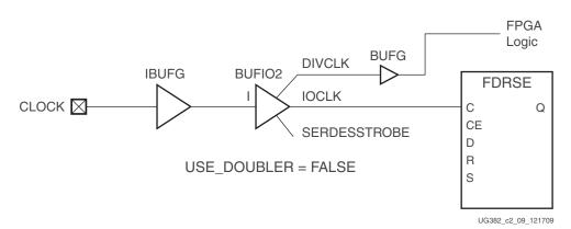
Figure 1-12: I/O Flip-Flop Clocking using BUFIO2
