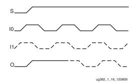
Figure 1-24: BUFGMUX\_1 (CLK\_SEL\_TYPE = SYNC) Timing Diagram
