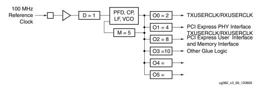
Figure 3-7: PLL as a Frequency Synthesizer
