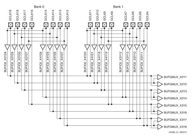
A graphical representation of the conflicting BUFGMUX inputs is shown in Figure 1-3 and Figure 1-4.
