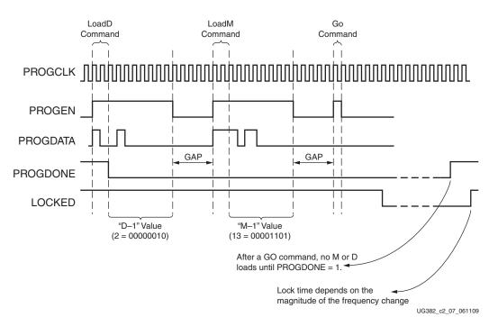
Figure 2-14: DCM\_CLKGEN M and D Configuration Timing Waveform
