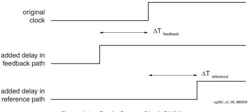
Figure 3-9: Basic Output Clock Shifting
