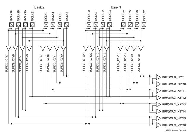
Figure 1-4: BUFGMUX Connections for Bank 2 and Bank 3
