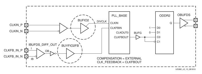
Figure 3-14: Zero Delay Buffer for Differential Clocks
