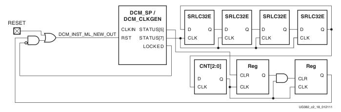
Figure 2-12: Low-Power Reset Circuit
