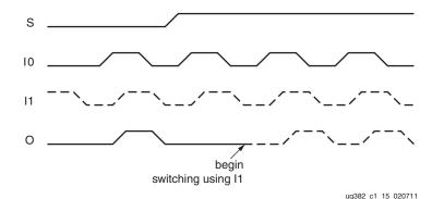
Figure 1-23: BUFGMUX (CLK\_SEL\_TYPE = SYNC) Timing Diagram
