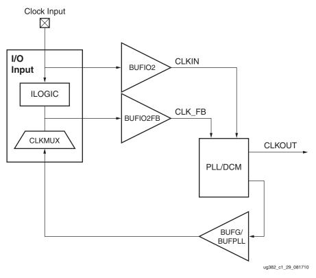
Figure 1-40: BUFIO2FB Buffer Matches Clock Routing Delay
