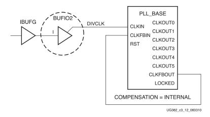
Figure 3-12: PLL with Internal Feedback
