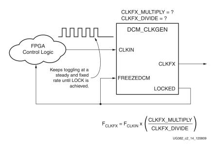
Figure 2-20: Setup of a Free-Running Oscillator
