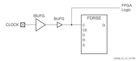
Figure 1-13: I/O Flip-Flop Clocking using BUFG
