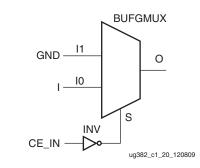
Figure 1-28: Equivalent Functionality of BUFGCE
