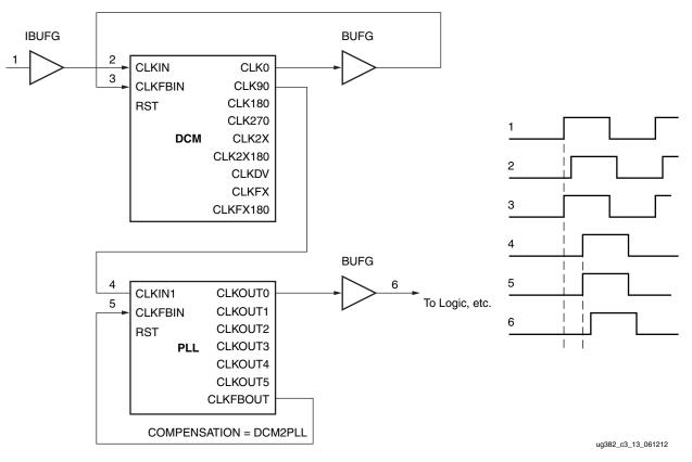
Figure 3-15: DCM Driving a PLL
