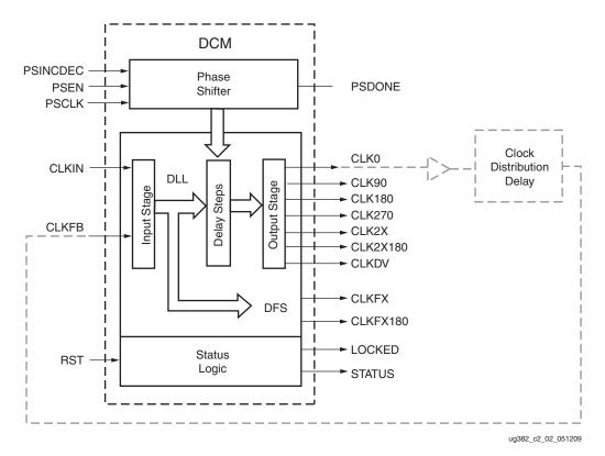
The DCM consists of four distinct functions that can operate independently or in tandem. Figure 2-2 shows a simplified block diagram of a DCM.
