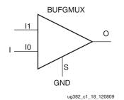
Figure 1-26: BUFG Built from a BUFGMUX
