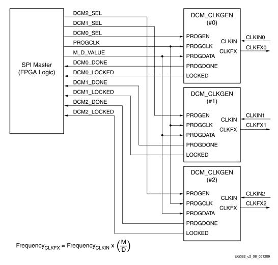
*Figure 2-13:* **DCM\_CLKGEN M and D Programming Interface**
