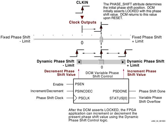
Figure 2-7: Variable Phase Shift With PHASE\_SHIFT ≠ 0
