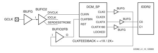
Figure 1-18: Example 5: DCM Deskewed to the Inputs
