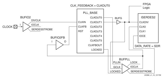
Figure 1-16: Example 3: Basic PLL ISERDES2 (SDR)
