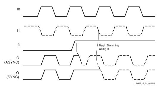
Figure 1-22: BUFGMUX ASYNC vs. SYNC Timing Diagram
