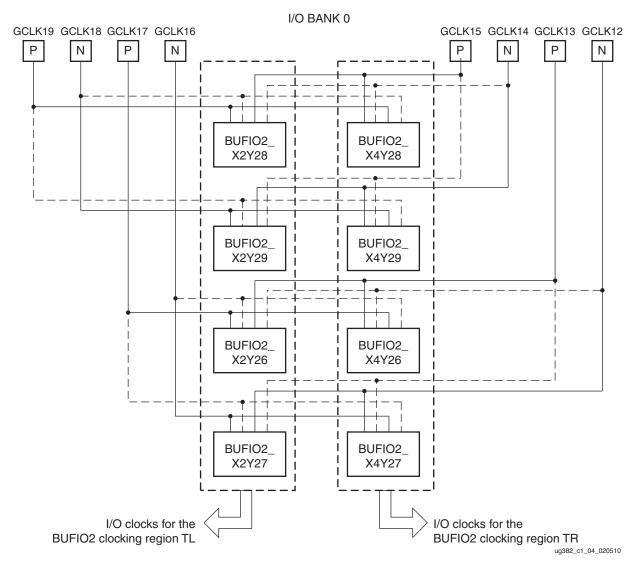
Figure 1-7: I/O Clock Spanning a Full Bank
