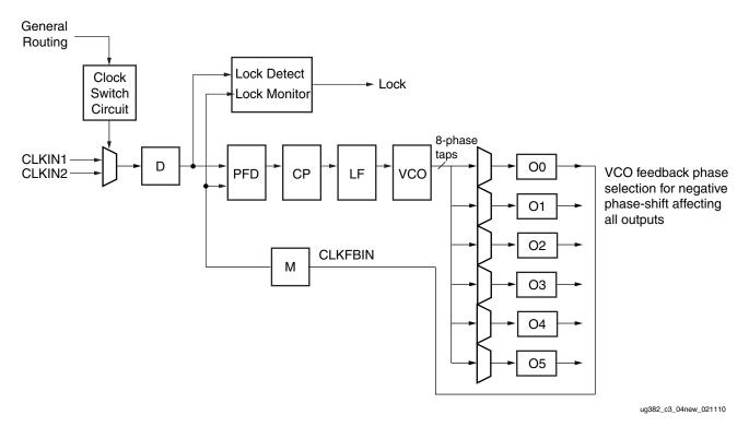
*Figure 3-4:* **Detailed PLL Block Diagram: CLK\_FEEDBACK = CLKOUT0**
