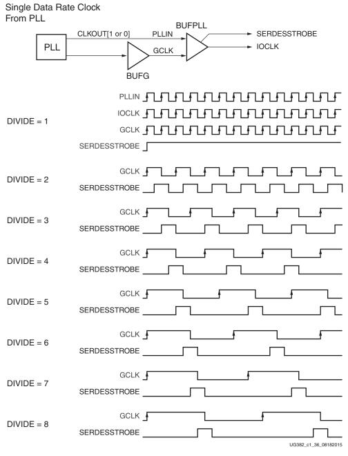
Figure 1-38: BUFPLL Single Data Rate Clock
