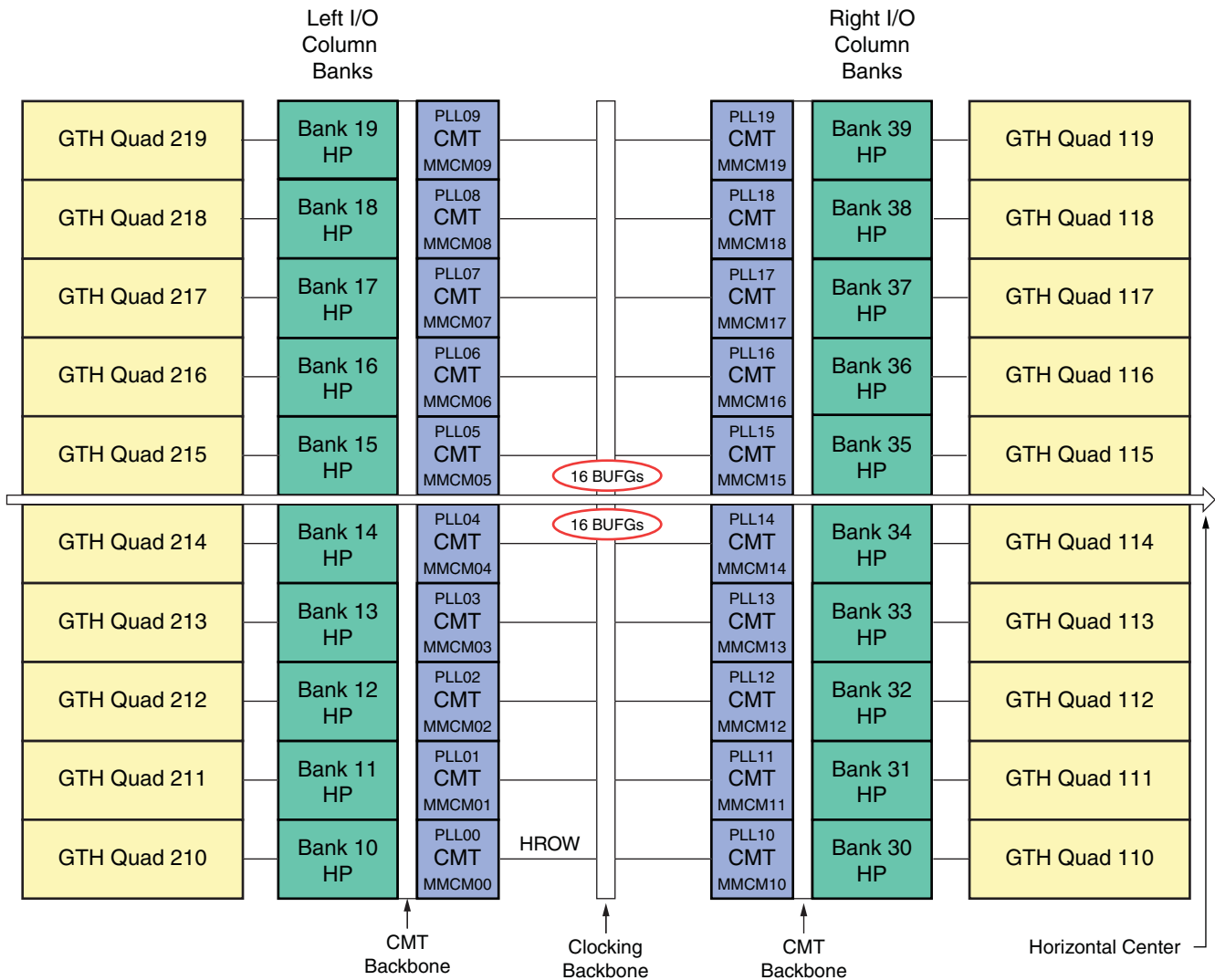
Figure 1-24: XC7VX690T and XQ7VX690T Banks
