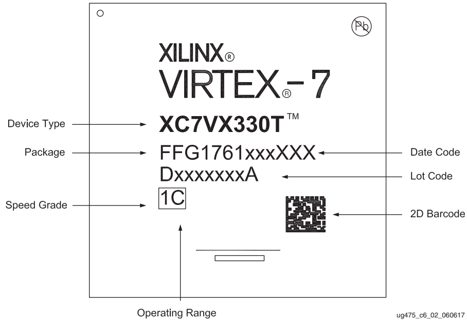
Figure 6-4: Virtex-7 Device Package Marking
