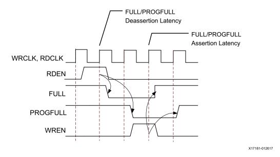
Figure 1-29: Deassertion and Assertion Latencies of FULL and PROGFULL for Common-Clock FIFO
