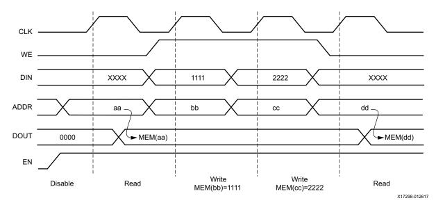
Figure 1-4: NO\_CHANGE Mode Waveforms
