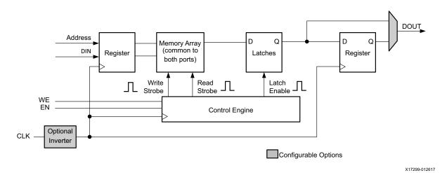
Figure 1-5: Block RAM Logic Diagram (One Port Shown)
