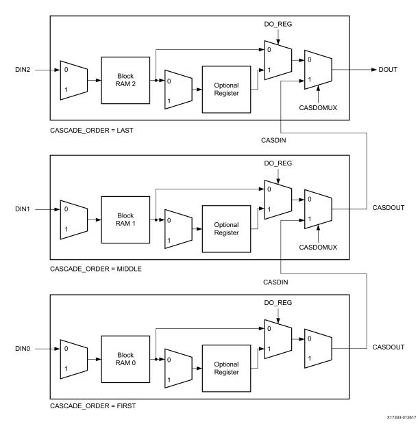
Figure 1-9: Block RAM Cascade – Standard Data Out Cascade
