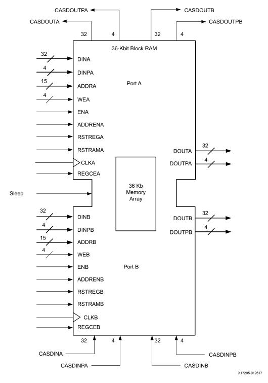
Figure 1-1: RAMB36 Usage in a True Dual-Port Data Flow
