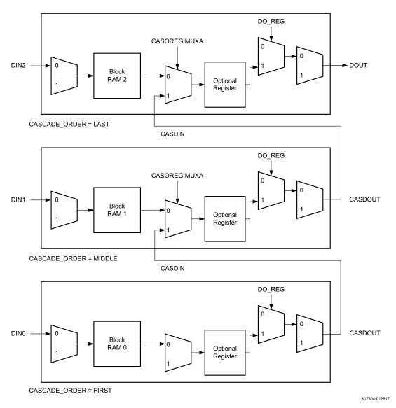
Figure 1-10: Block RAM Cascade - Pipelined Data Out Cascade
