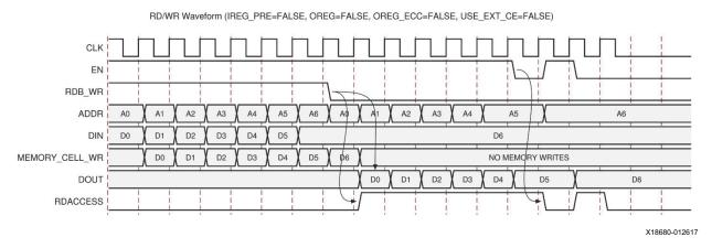
Figure 2-9: Read/Write with Attributes IREG\_PRE\_A/B=FALSE, OREG\_ECC\_A/B=FALSE, USE\_EXT\_CE\_A/B=FALSE
