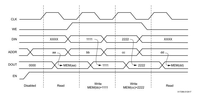
Figure 1-2: WRITE\_FIRST Mode Waveforms
