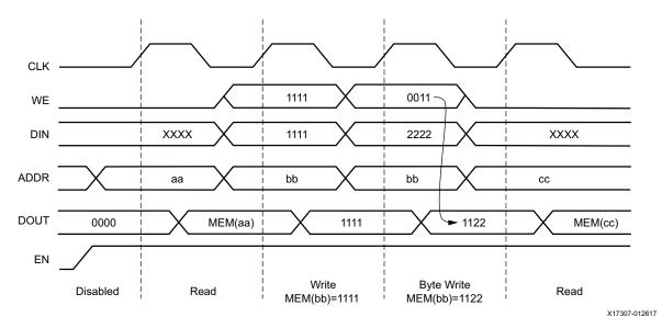
Figure 1-13: Byte-wide Write Operation Waveforms (x36 WRITE\_FIRST)
