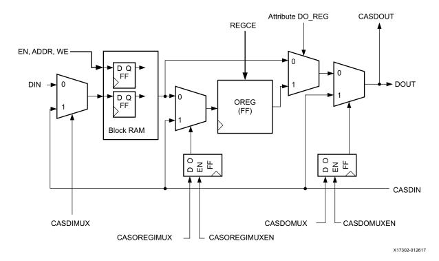
Figure 1-8: Cascade Functional Diagram
