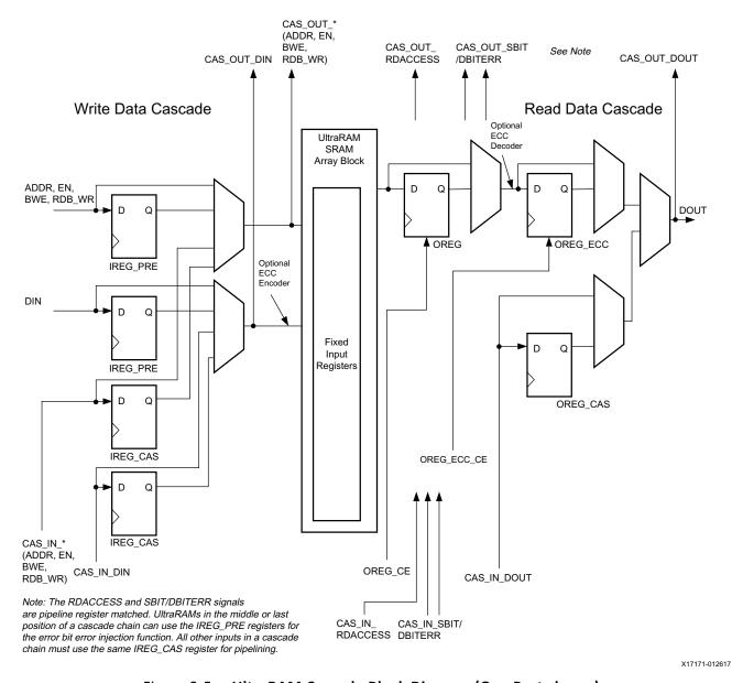
Figure 2-5: UltraRAM Cascade Block Diagram (One Port shown)
