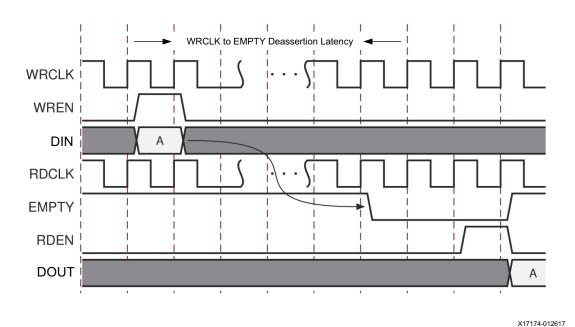
Figure 1-23: Standard FIFO Interface
