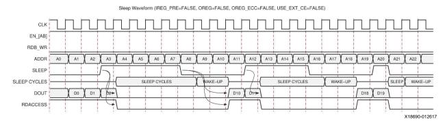
Figure 2-19: Sleep Mode for Read Operations With Attributes IREG\_PRE\_A/B=FALSE, OREG\_A/B= FALSE, OREG\_ECC\_A/B= FALSE, USE\_EXT\_CE\_A/B= FALSE, DOUT is Forced to "0"
