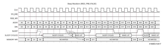
Figure 2-18: Sleep Mode for Write Operations With Attribute IREG\_PRE\_A/B=FALSE
