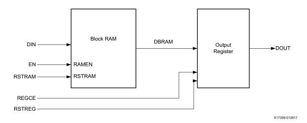
Figure 1-16: Block RAM RSTREG in Register Mode
