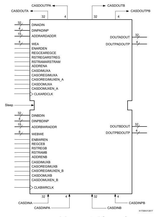
Figure 1-14: Block RAM Port Signals (RAMB36E2)
