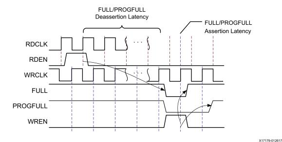
Figure 1-27: Deassertion and Assertion Latencies of FULL and PROGFULL for Independent-Clock FIFO
