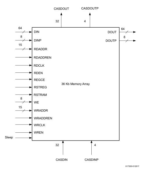
Figure 1-6: RAMB36 Usage in a Simple Dual-Port Data Flow
