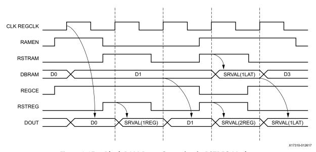
Figure 1-17: Block RAM Reset Operation in RSTREG Mode
