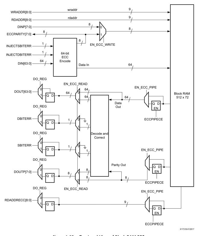
Figure 1-32: Top-Level View of Block RAM ECC
