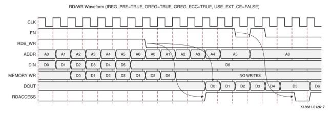
Figure 2-10: Reset/Read/Write with Attributes IREG\_PRE\_A/B=TRUE, OREG\_ECC\_A/B=TRUE, USE\_EXT\_CE\_A/B=FALSE
