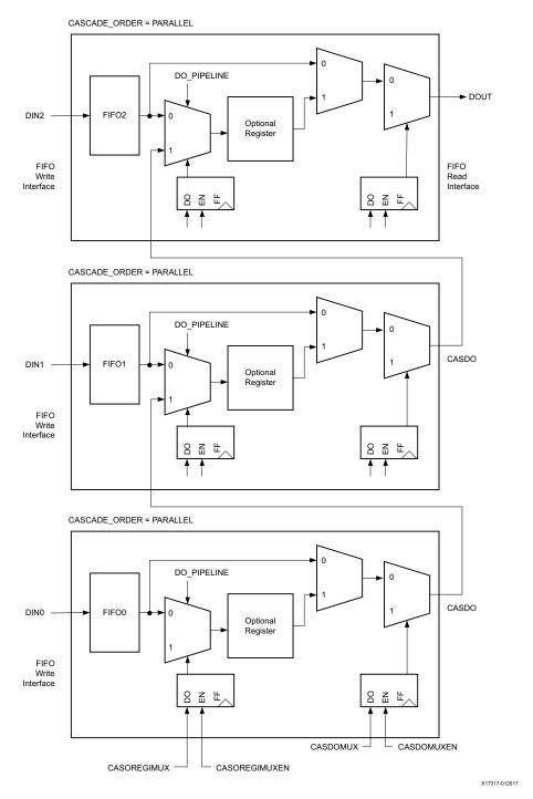
Figure 1-31: FIFO Parallel Cascade
