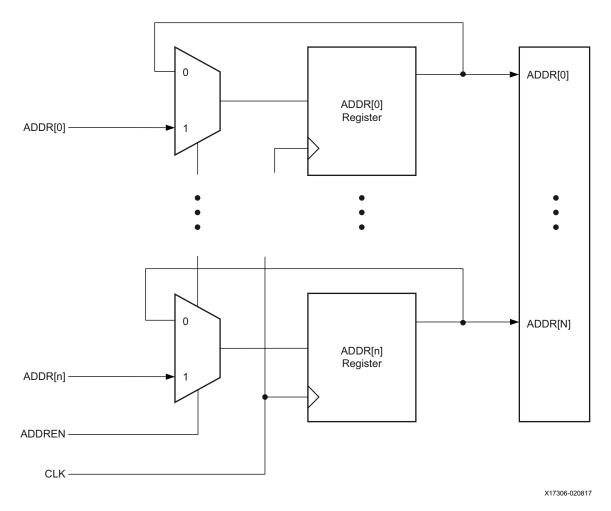
Figure 1-12: Address Latching Enable
