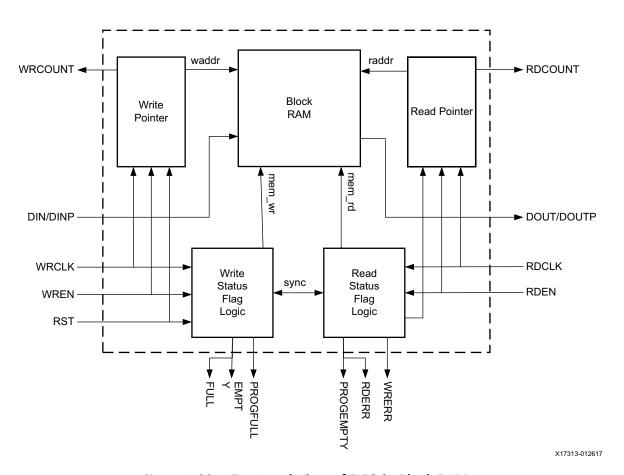
Figure 1-20: Top-Level View of FIFO in Block RAM
