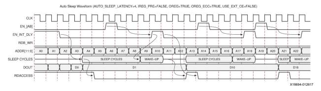
Figure 2-24: Auto Sleep Mode for Read Operations With Attributes AUTO\_SLEEP\_LATENCY=4, IREG\_PRE\_A/B=FALSE, OREG\_A/B= TRUE, OREG\_ECC\_A/B= TRUE, USE\_EXT\_CE\_A/B= FALSE
