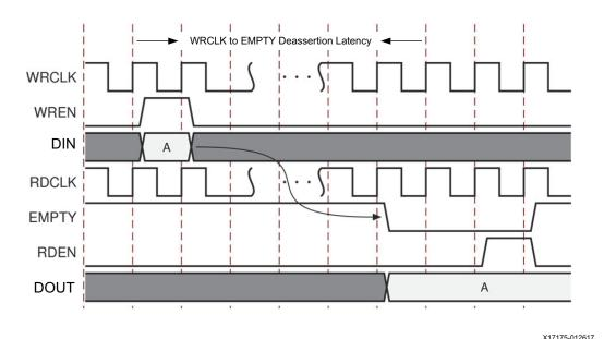
Figure 1-24: FWFT FIFO with One Data Word in the FIFO
