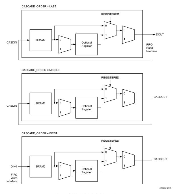
Figure 1-30: FIFO Serial Cascade
