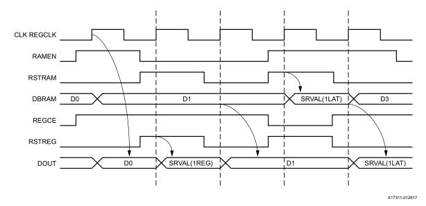
Figure 1-18: Block RAM Reset Operation in REGCE Mode
