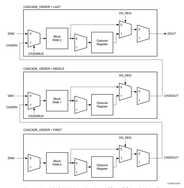
Figure 1-11: Block RAM Cascade – Arrayed (Systolic) Data in Cascade
