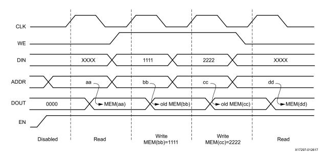
Figure 1-3: READ\_FIRST Mode Waveforms
