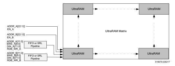
Figure 2-23: Typical Fabric Implementation for Using Auto Sleep Mode
