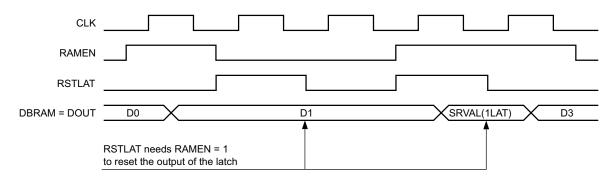
Figure 1-19: Block RAM Reset Operation in Latch Mode
