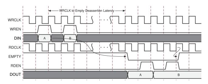
Figure 1-25: FWFT FIFO with Two Data Words in the FIFO
