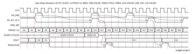
Figure 2-27: Auto Sleep Mode for Read Operations With Attributes AUTO\_SLEEP\_LATENCY=8, IREG PRE A/B=FALSE, OREG A/B= TRUE, OREG ECC A/B= FALSE, USE EXT CE A/B= FALSE
