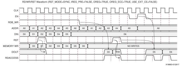
Figure 2-12: Reset/Read/Write with Attributes RST\_MODE=SYNC, IREG\_PRE\_A/B=FALSE, OREG\_A/B=TRUE, OREG\_ECC\_A/B=TRUE, USE\_EXT\_CE\_A/B=FALSE
