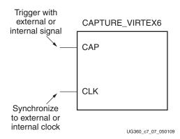
Figure 7-6: Virtex-6 FPGA Library Primitive
