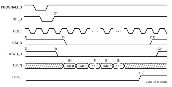
Figure 2-8: Continuous x8 SelectMAP Data Loading
