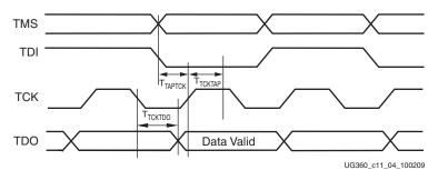
Figure 11-4: Virtex-6 FPGA Boundary-Scan Port Timing Waveforms
