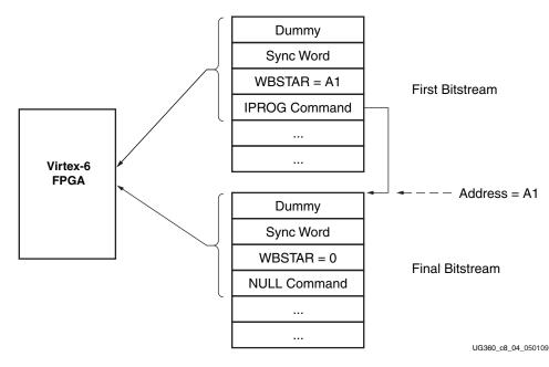
Figure 8-4: IPROG Embedded in the Bitstream
