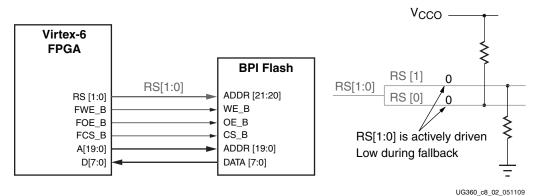
Figure 8-2: Fallback Reconfiguration Usage for BPI
