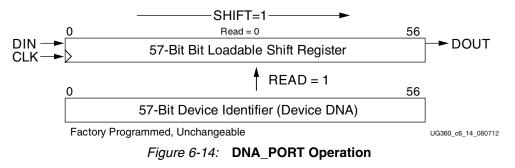
To read the Device DNA, the FPGA application must first transfer the identifier value into the DNA\_PORT output shift register. The READ input must be asserted during a rising
