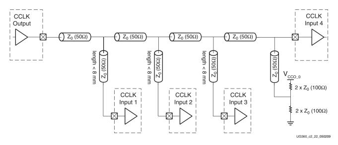
Figure 2-21: Multi-Drop: One CCLK Output, More Than Two CCLK Inputs
