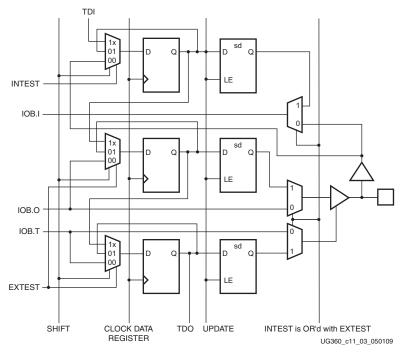
Figure 11-3: Virtex-6 FPGA Boundary-Scan Logic
