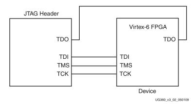
Figure 3-2: Single Device JTAG Programming Connections
