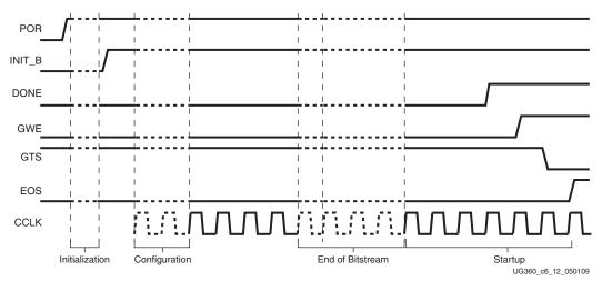
Figure 6-12: Configuration Signal Sequencing (Default Startup Settings)
