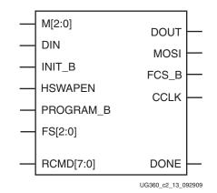
Figure 2-11: Virtex-6 FPGA SPI Configuration Interface
