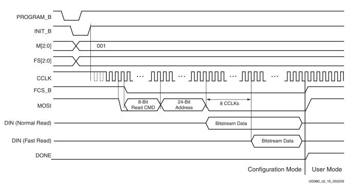
The Virtex-6 FPGA SPI flash timing diagram is shown in Figure 2-13.
