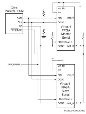
Configuration can be driven from a configuration PROM or from an external configuration controller.
