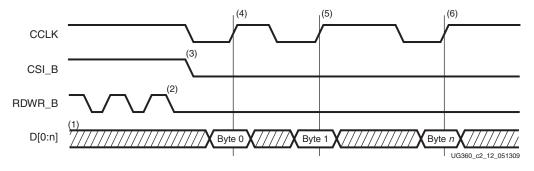
Figure 2-10: Non-Continuous SelectMAP Data Loading with Controlled CCLK
