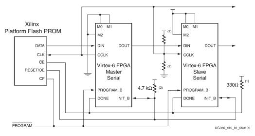
Figure 10-1: Master/Slave Serial Mode Daisy Chain Configuration
