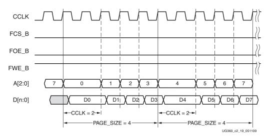
Figure 2-17: BPI-Up Waveforms (Page Size = 4 and First Access CCLK = 2)
