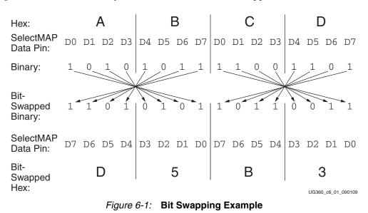
Figure 6-1 shows how two bytes of data (0xABCD) are bit swapped.
