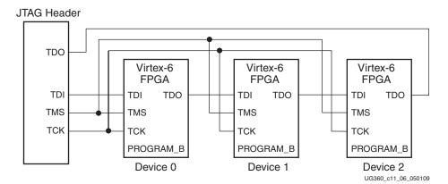
Figure 11-6: Boundary-Scan Chain of Devices
