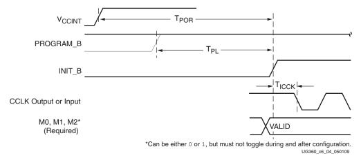
Figure 6-4: Device Power-Up Timing
