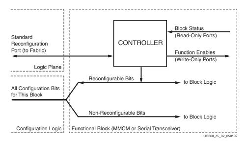
Figure 5-2: Block Configuration Logic with Dynamic Interface
