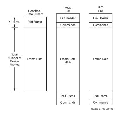
Figure 7-5: Comparing Readback Data Using the MSK and BIT Files
