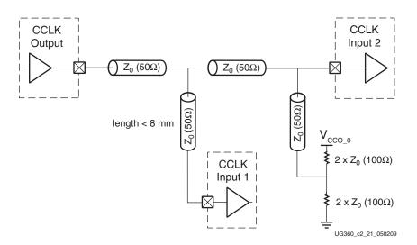
Figure 2-20: Multi-Drop: One CCLK Output, Two CCLK Inputs
