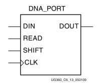
Figure 6-13: Virtex-6 FPGA DNA\_PORT Design Primitive
