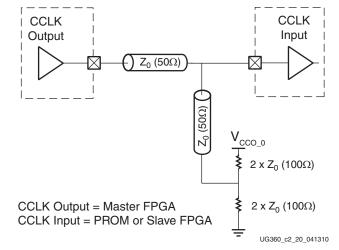
Figure 2-19: Point-to-Point: One CCLK Output, One CCLK Input
