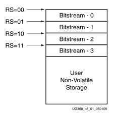
Figure 8-1: BPI Flash Address Space for MultiBoot
