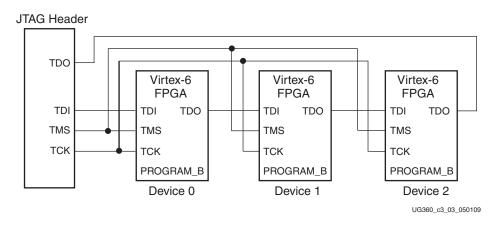
Figure 3-3: Boundary-Scan Chain of Devices
