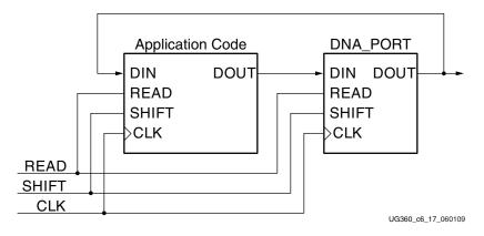
Figure 6-17: Bitstream Specific Code
