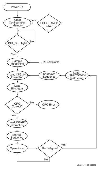
Figure 11-5: Device Configuration Flow Diagram
