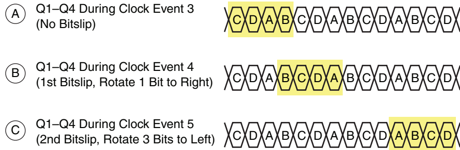
Figure 3-17: Bits from Data Input Stream (D) of Figure 3-16
