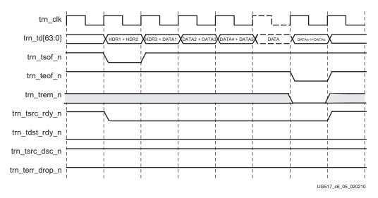
Figure 6-5: TLP with 3-DW Header with Payload
