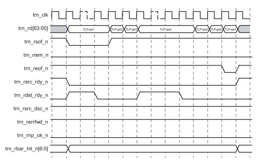
Figure 6-18: User Application Throttling Receive TLP
