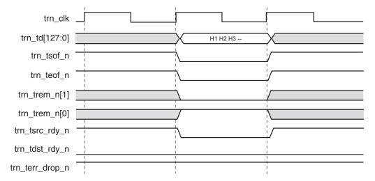
Figure 6-27: TLP 3-DW Header without Payload
