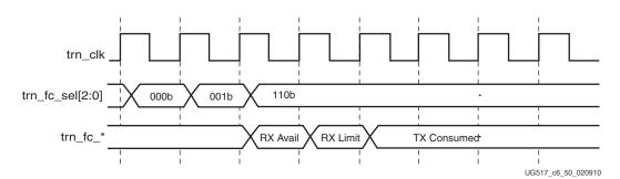
Figure 6-50: Flow Control Credits for 64-bit Interface
