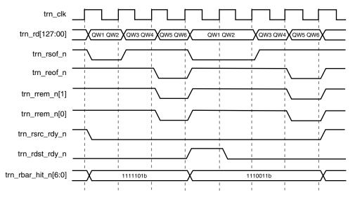
Figure 6-48: BAR Target Determination using trn\_rbar\_hit
