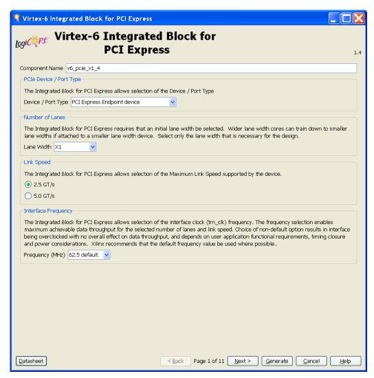
Figure 5-1: Screen 1: Integrated Block for PCI Express Parameters
