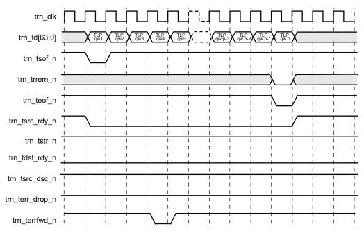
Figure 6-12: Packet Data Poisoning on the Transmit Transaction Interface
