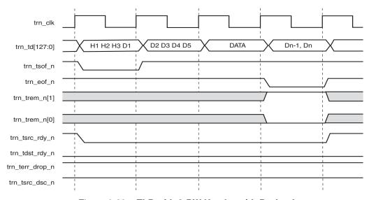
Figure 6-29: TLP with 3-DW Header with Payload
