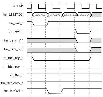
Figure 6-36: Packet Data Poisoning on the Transmit Transaction Interface
