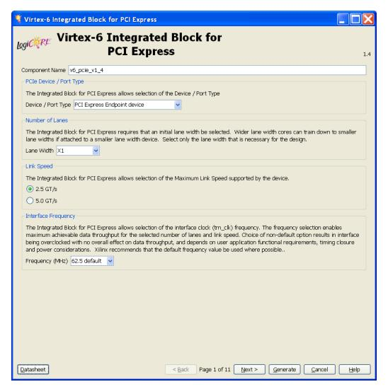
Figure 4-7: Integrated Block Main Screen
