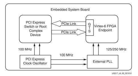
Figure 6-65: Embedded System Using 125/250 MHz Reference Clock
