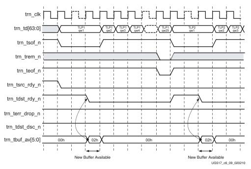
Figure 6-9: Destination Throttling of the Endpoint Transmit Transaction Interface
