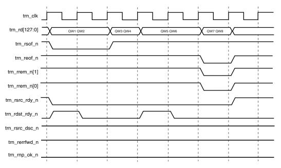
Figure 6-42: User Application Throttling Receive TLP
