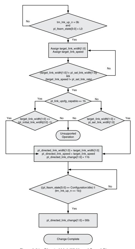
Figure 6-54: Directed Link Width and Speed Change
