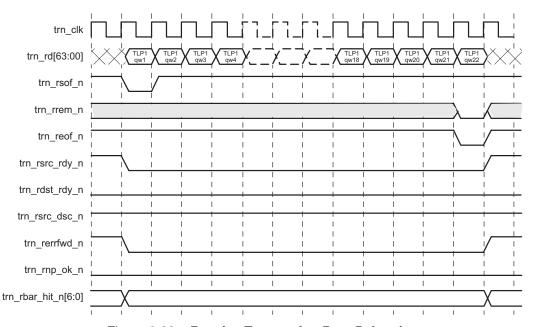
Figure 6-22: Receive Transaction Data Poisoning
