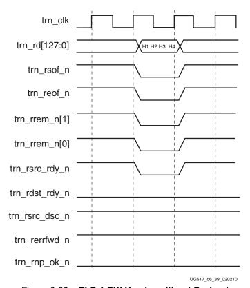
Figure 6-39: TLP 4-DW Header without Payload
