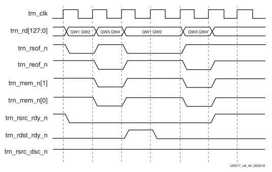
Figure 6-44: User Application Throttling Back-to-Back TLPs
