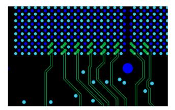
Figure F-4: Transmit Breakout Pattern
