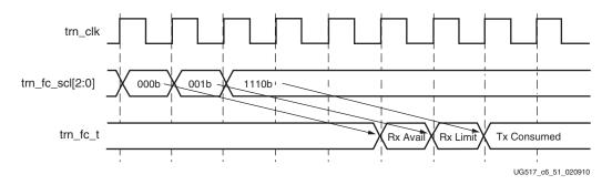
Figure 6-51: Flow Control Credits for 128-bit Interface
