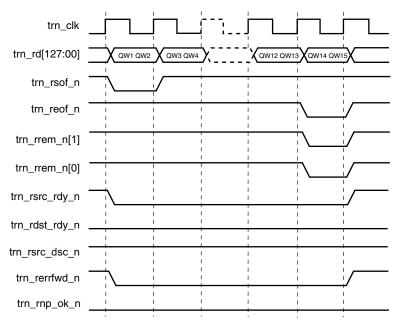
Figure 6-47: Receive Transaction Data Poisoning
