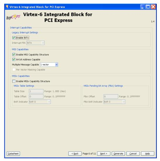
Figure 5-8: Screen 6: Interrupt Capabilities
