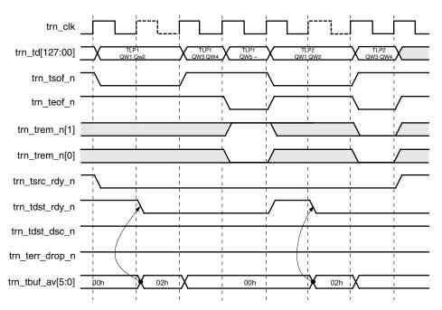
Figure 6-33: Destination Throttling of the Endpoint Transmit Transaction Interface
