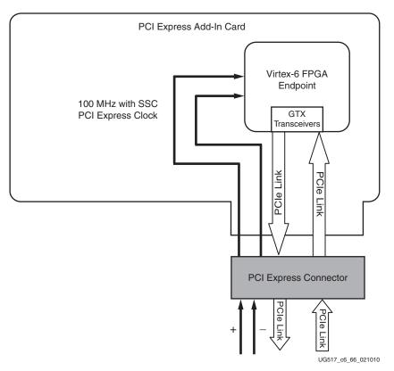
Figure 6-66: Open System Add-In Card Using 100 MHz Reference Clock
