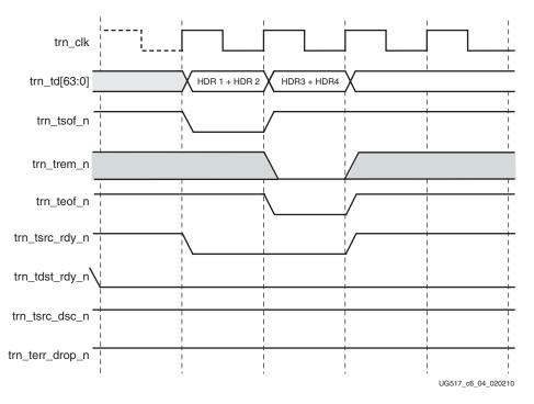
Figure 6-4: TLP with 4-DW Header without Payload
