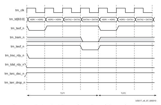
Figure 6-7: Back-to-Back Transaction on Transmit Transaction Interface
