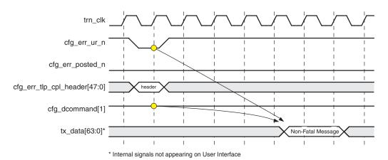
Figure 6-59: Signaling Unsupported Request for Posted TLP
