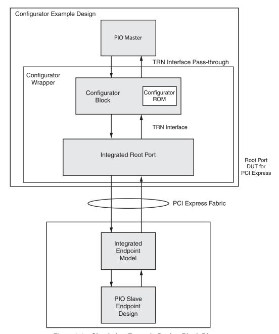
Figure 4-4: Simulation Example Design Block Diagram
