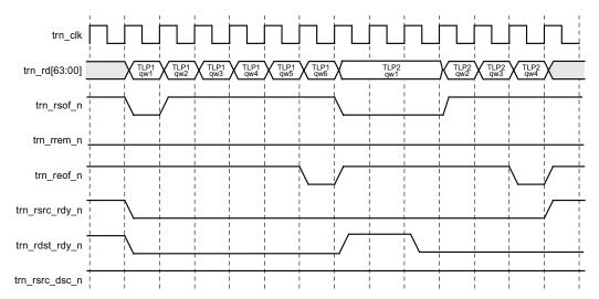
Figure 6-20: User Application Throttling Back-to-Back TLPs
