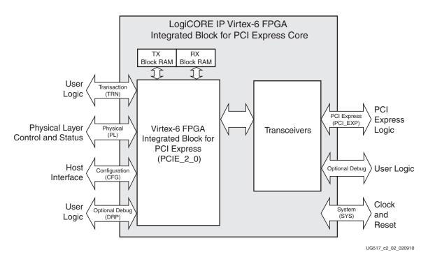
Figure 2-1: Top-Level Functional Blocks and Interfaces
