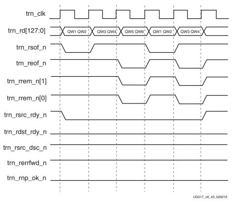
Figure 6-43: Receive Back-to-Back Transactions
