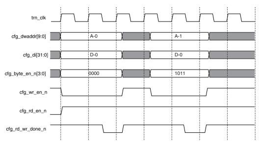
Figure 6-56: Example Configuration Space Write Access
