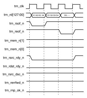
Figure 6-41: TLP 4-DW Header with Payload
