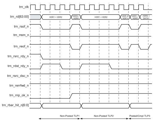
Figure 6-21: Packet Re-ordering on Receive Transaction Interface
