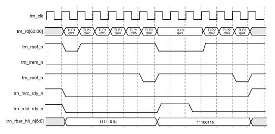
Figure 6-23: BAR Target Determination using trn rbar hit
