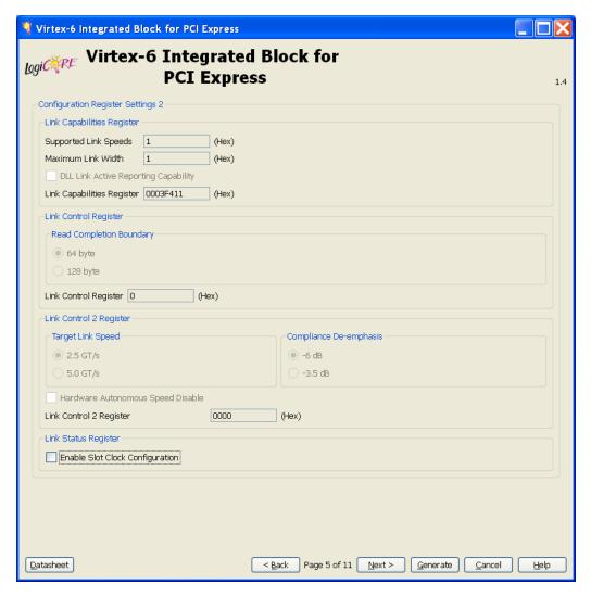
Figure 5-6: Screen 5: Configuration Settings
