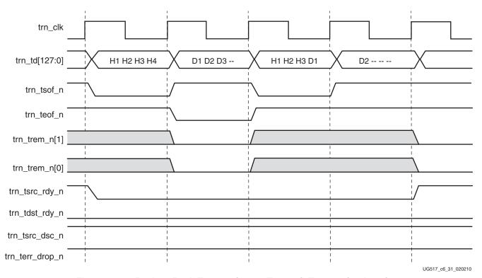
Figure 6-31: Back-to-Back Transaction on Transmit Transaction Interface
