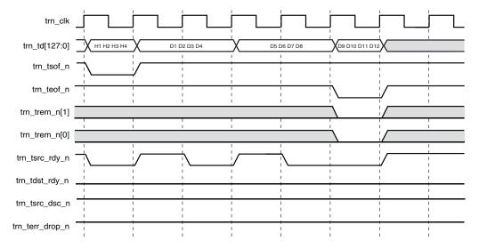
Figure 6-32: Source Throttling on the Transmit Datapath
