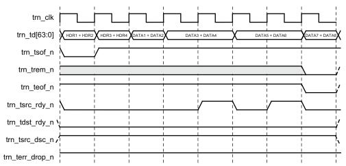
Figure 6-8: Source Throttling on the Transmit Datapath
