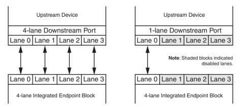
Figure 6-63: Scaling of 4-Lane Endpoint Core from 4-Lane to 1-Lane Operation
