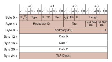
Figure 6-25: PCI Express Base Specification Byte Order
