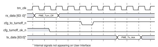
Figure 6-61: Power Management Handshaking: 64-bit
