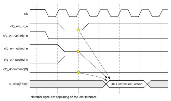
Figure 6-60: Signaling Locked Unsupported Request for Locked Non-Posted TLP
