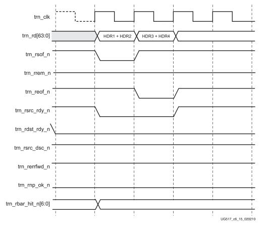
Figure 6-15: TLP 4-DW Header without Payload
