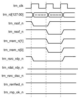
Figure 6-40: TLP 3-DW Header with Payload
