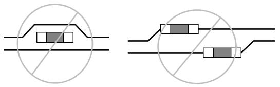
Figure F-5: Non-Symmetrical Routing Examples
