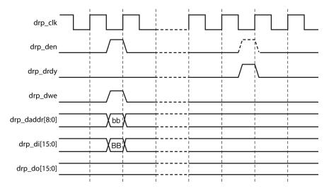
Figure 6-68: DRP Interface Write Cycle
