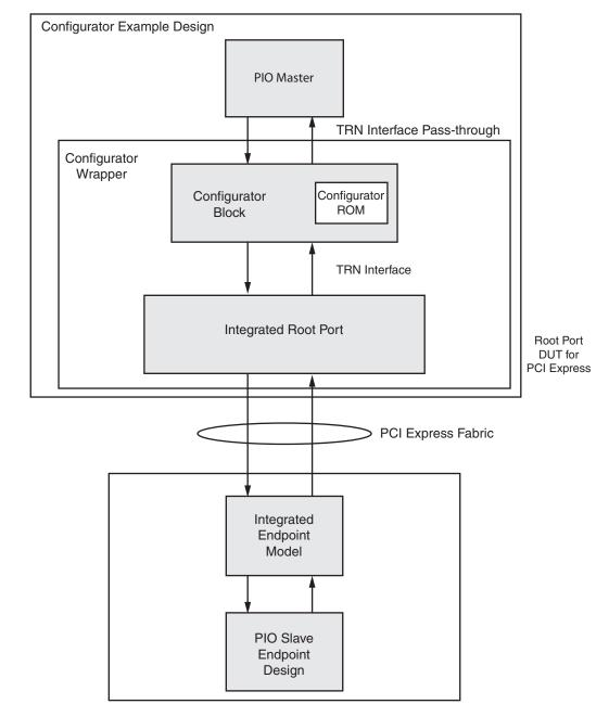
Figure B-2 shows how the blocks are connected in an overall system view.
