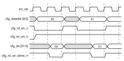
Figure 6-55: Example Configuration Space Read Access
