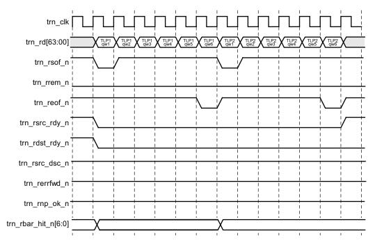
Figure 6-19: Receive Back-to-Back Transactions
