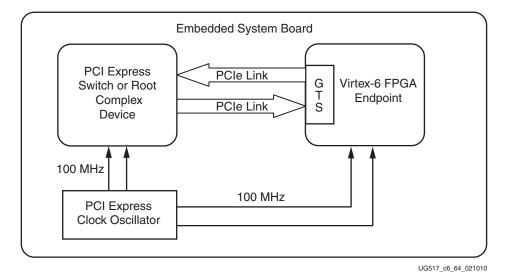
Figure 6-64: Embedded System Using 100 MHz Reference Clock
