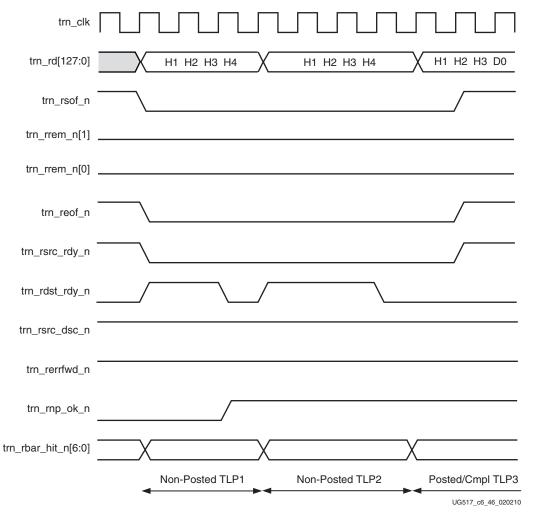
Figure 6-46: Packet Re-ordering on Receive Transaction Interface
