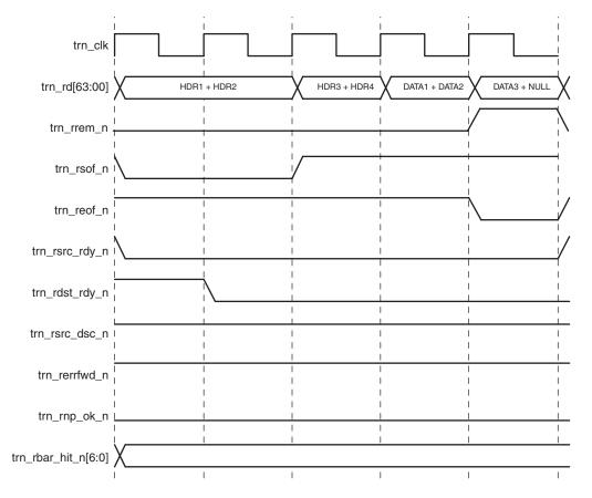
Figure 6-17: TLP 4-DW Header with Payload
