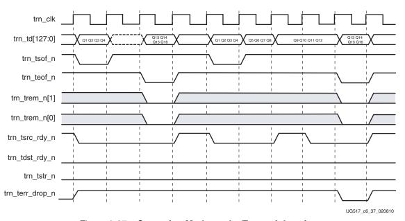
Figure 6-37: Streaming Mode on the Transmit Interface
