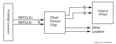
Figure F-7: Fanout Block Diagram
