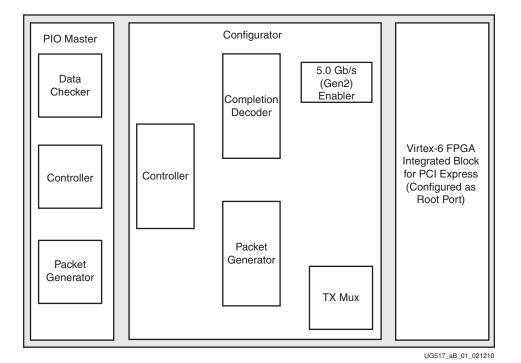
Figure B-1: Configurator Example Design Components
