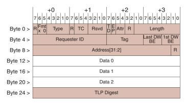
Figure 6-1: PCI Express Base Specification Byte Order
