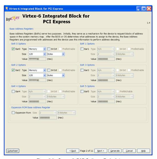
Figure 5-2: Screen 2: BAR Options - Endpoint
