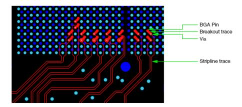
Figure F-3: Receive Breakout Pattern
