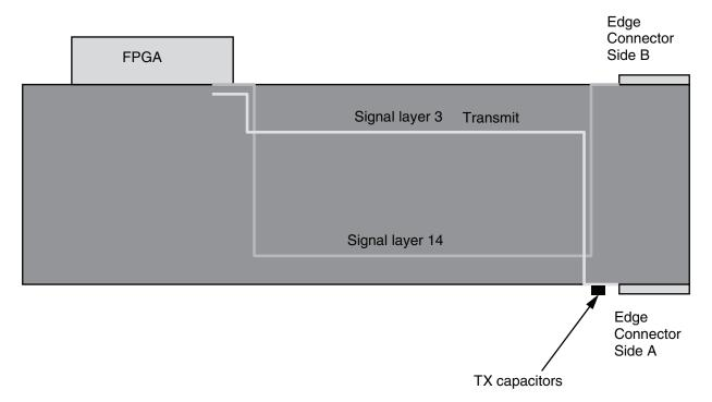
Figure F-2: Transmit and Receive Data Lines
