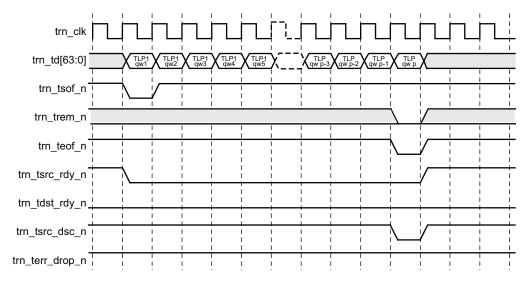
Figure 6-10: Source Driven Transaction Discontinue on Transmit Interface
