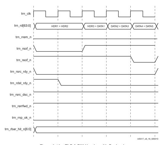
Figure 6-16: TLP 3-DW Header with Payload
