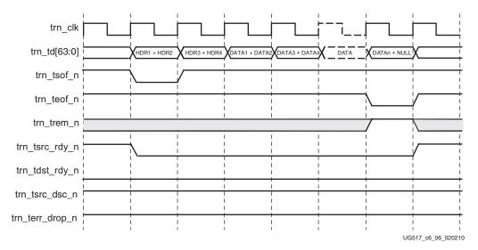
Figure 6-6: TLP with 4-DW Header with Payload
