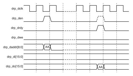
Figure 6-69: DRP Interface Read Cycle
