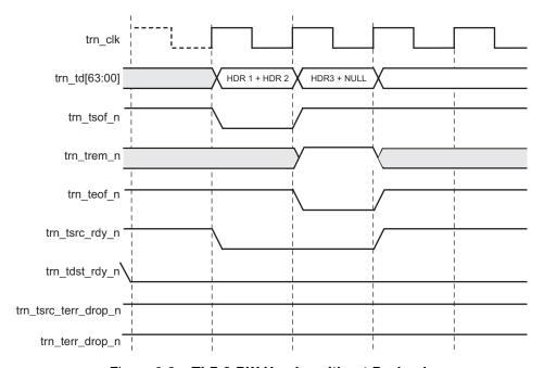
Figure 6-3: TLP 3-DW Header without Payload
