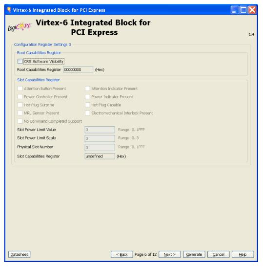
Figure 5-7: Screen 6: Configuration Settings
