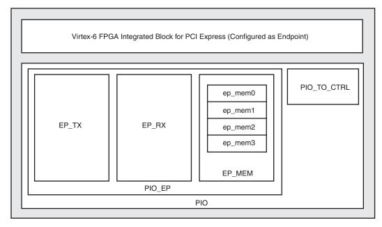
Figure 4-2: Implementation Example Design Block Diagram
