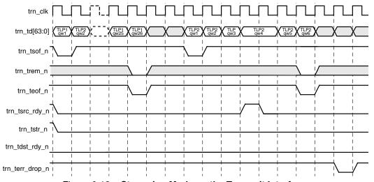
Figure 6-13: Streaming Mode on the Transmit Interface
