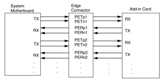
Figure F-6: Add-In Card Design Connections
