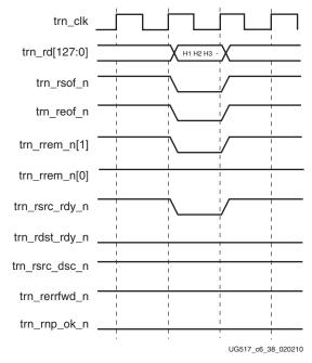
Figure 6-38: TLP 3-DW Header without Payload
