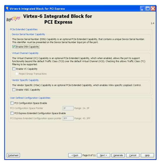
Figure 5-10: Screen 8: PCle Extended Capabilities
