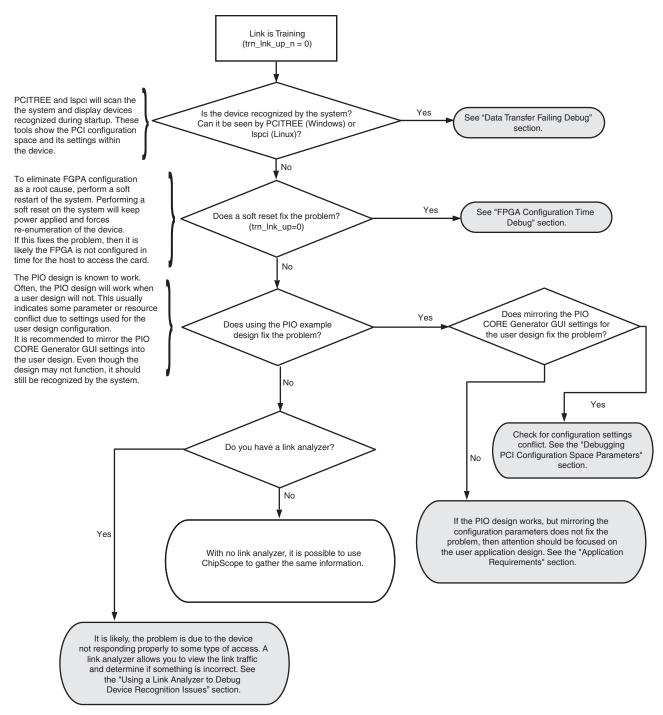
Figure D-4: Link Trained Debug Flow Diagram
