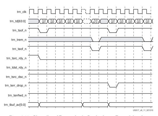
Figure 6-11: Discarding of Transaction by Destination on Transmit Interface
