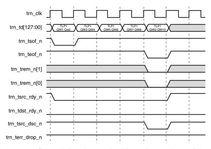
Figure 6-34: Source Driven Transaction Discontinue on Transmit Interface
