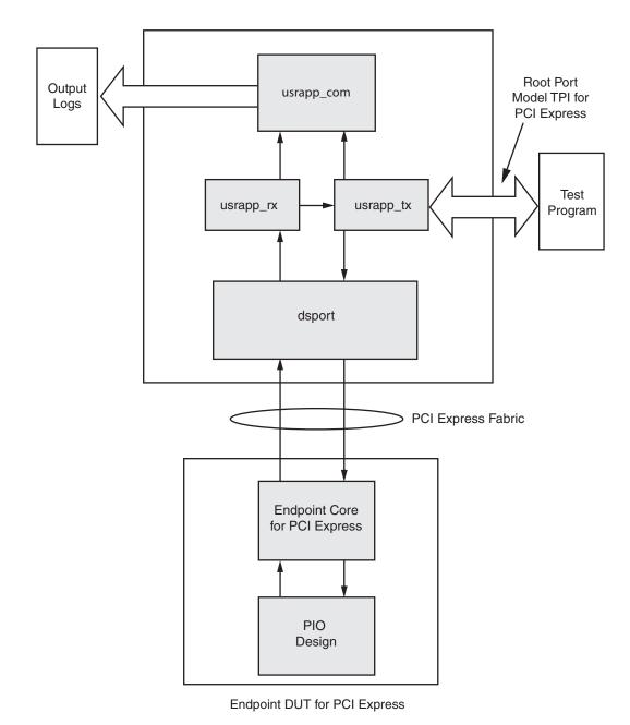
Figure 4-1: Simulation Example Design Block Diagram
