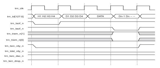
Figure 6-30: TLP with 4-DW Header with Payload
