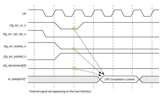
Figure 6-58: Signaling Unsupported Request for Non-Posted TLP
