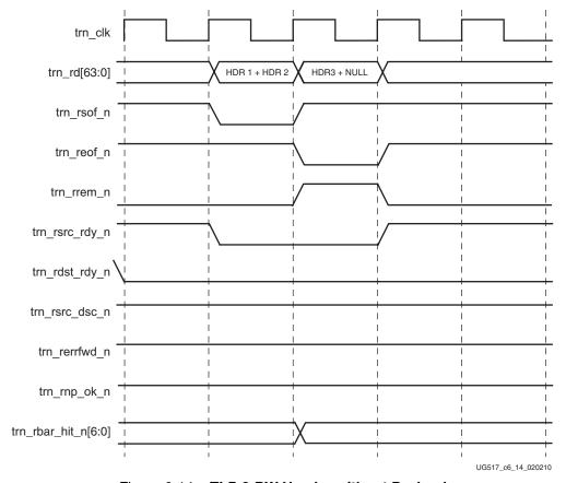
Figure 6-14: TLP 3-DW Header without Payload
