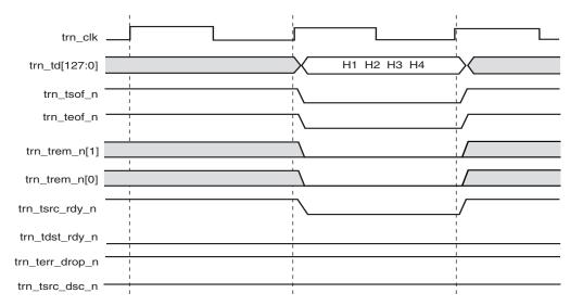
Figure 6-28: TLP with 4-DW Header without Payload
