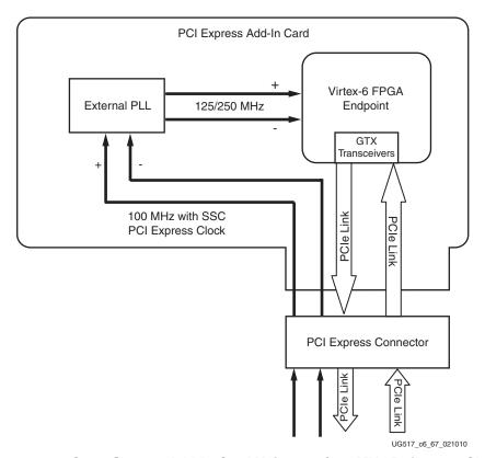
Figure 6-67: Open System Add-In Card Using 125/250 MHz Reference Clock
